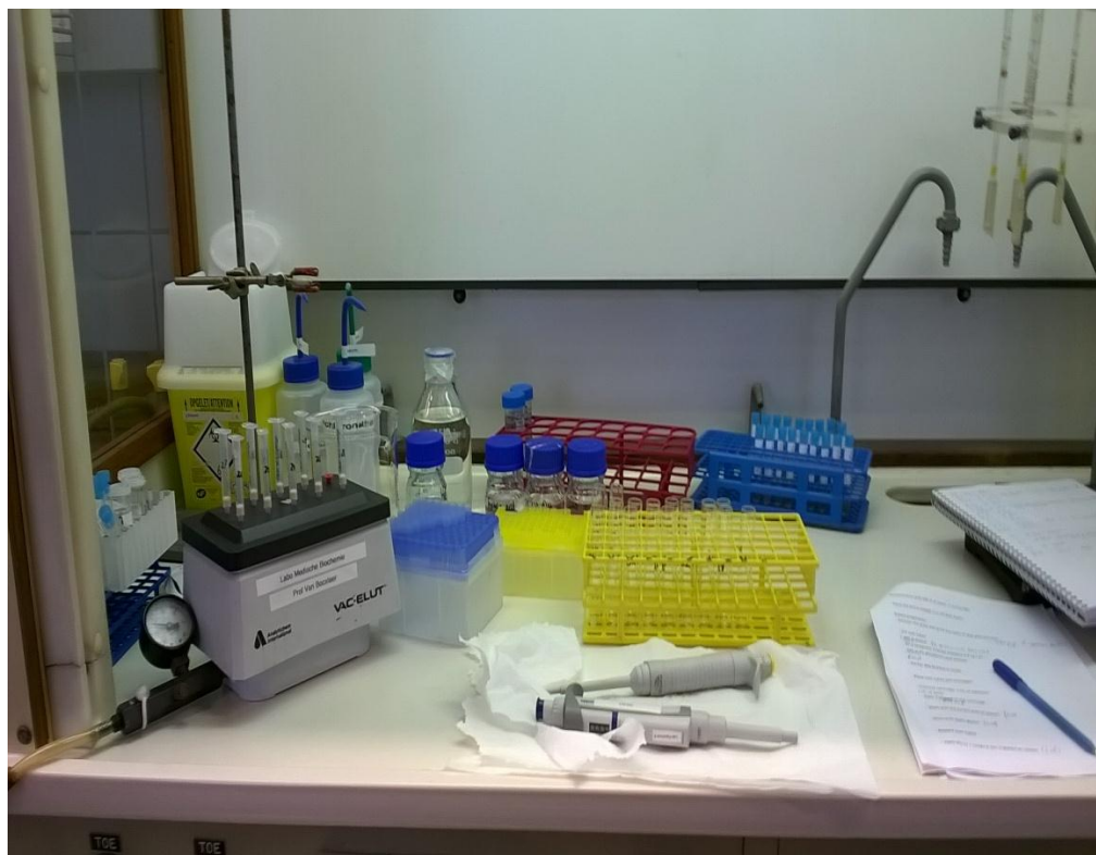
Plate V: Solid phase extraction of blood samples on a 10 port extraction manifold
