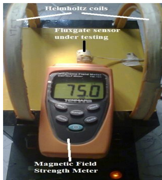
Plate 3.5: Actual Implemented Test-Bed (Helmholtz Coils) for Characterizing the FMS.
