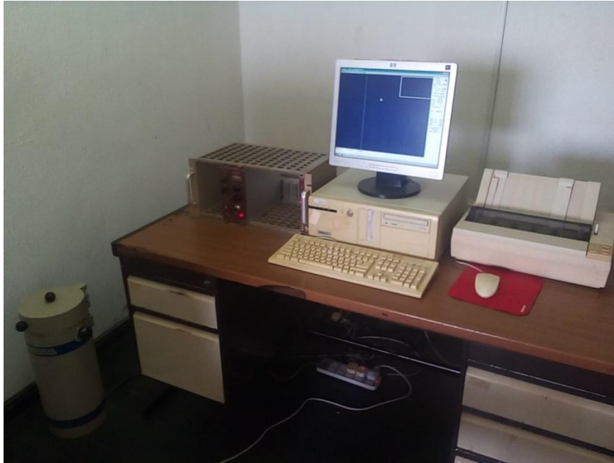
Plate VIII: Experimental Set up of the Gamma Spectrometry at Centre for Energy Research and Training, Ahmadu Bello University, Zaria
