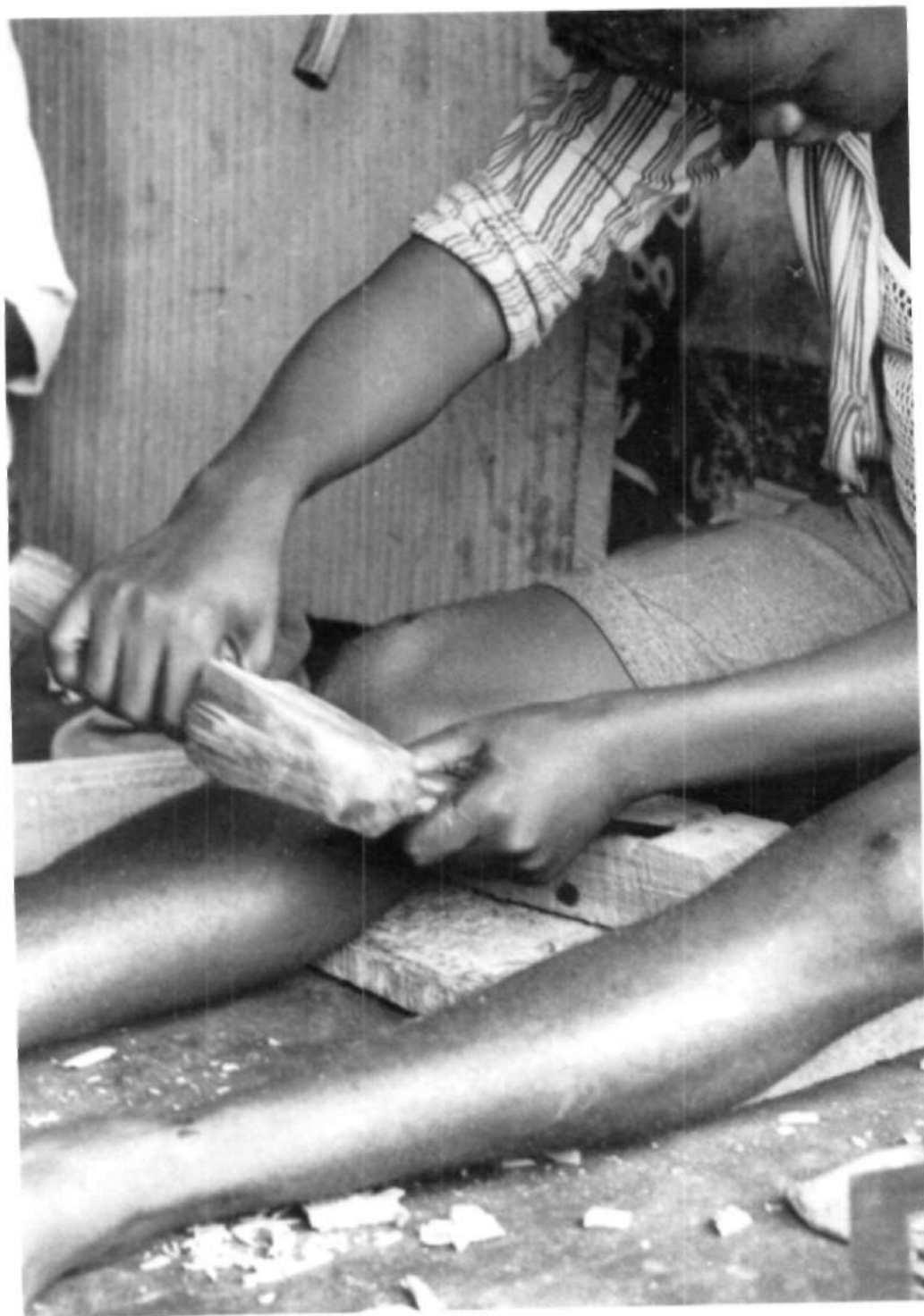
PLATE XXXIX. INCISING THE NECK LINE WITH A CHISEL
