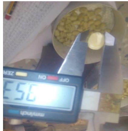
Plate C4: Seed width Determination
