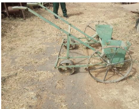
Plate 2.5. Two rows animal drawn seed Precision Planter (Isiaka et al. 2000)
