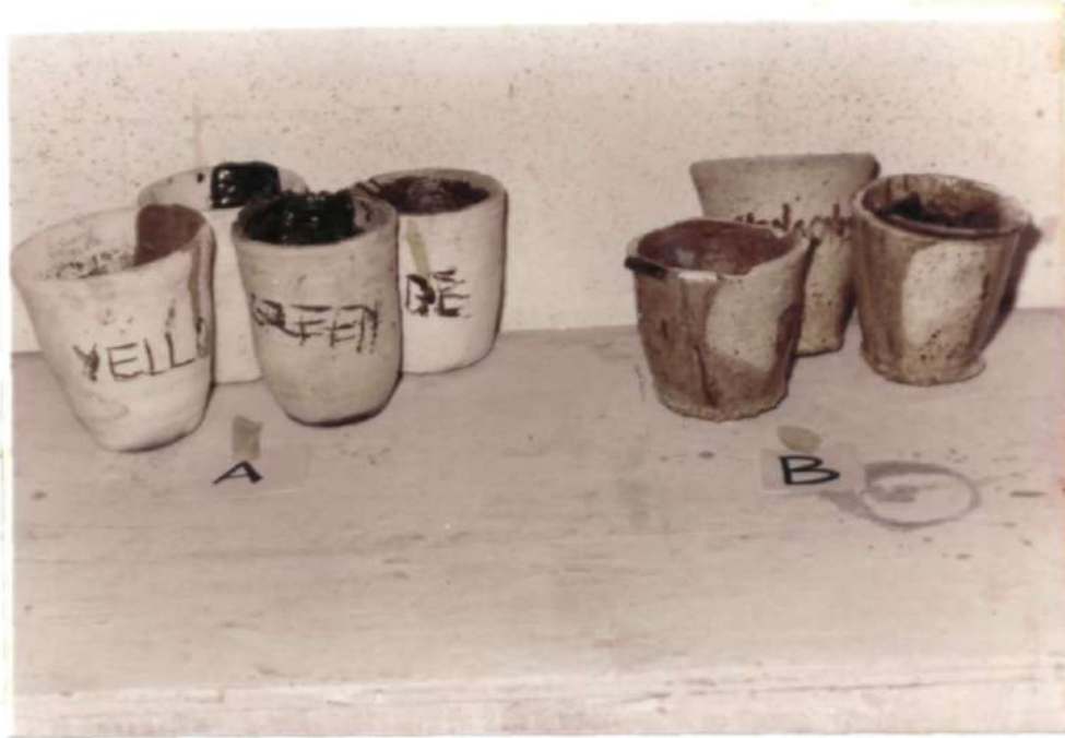
PLATE III: CRUCIBLES; 'A' Used for Melting Enamel 'B' Used for Melting Under-glaze Stain.
