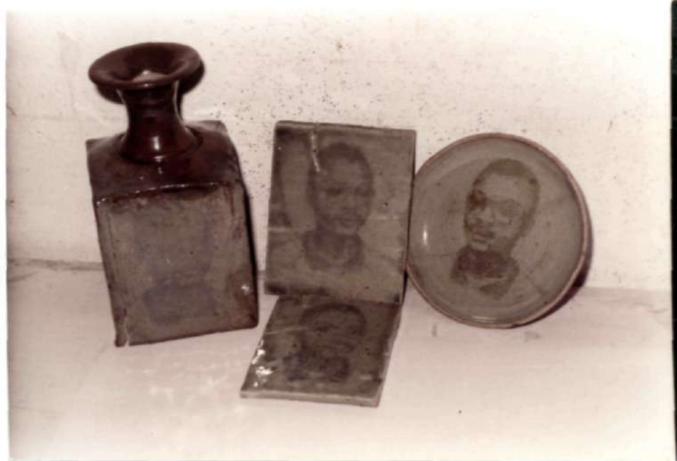
PLATE VIII: FIRED ENGOBE PRINTS SHOWING THE DIFFUSION OF THE INK INTO THE TRANSPARENT COVER GLAZE.
