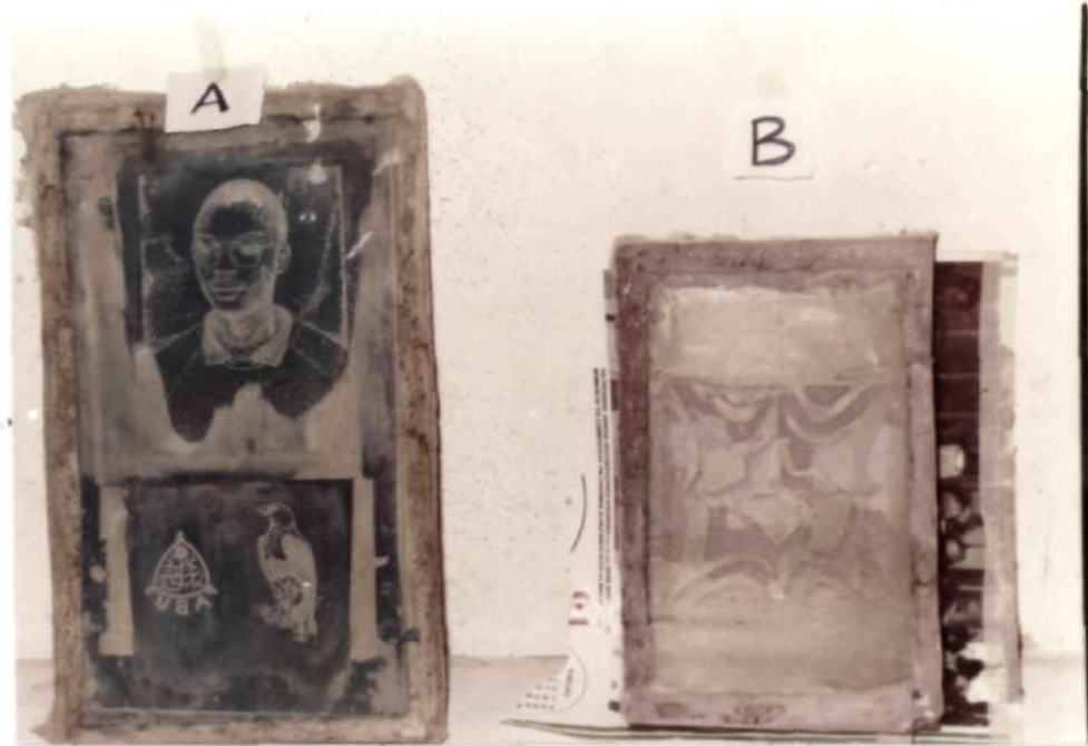
PLATE II: SCREENS: 'A' Photographic Stencil 'B' Lacquer Film Stencil.
