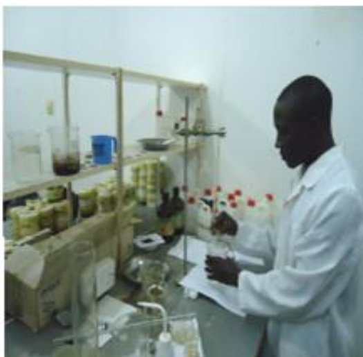
Plate VII, Researcher Titrating \text{Na}_2\text{SiO}_3(\text{aq}) against \text{Ca}(\text{NO}_3)_2(\text{aq}) + \text{HNO}_3(\text{conc})
