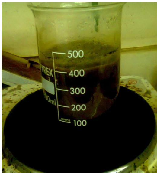
Plate V, Boiling solution of \text{RHA} + \text{NaOH}_{(\text{aq})}
