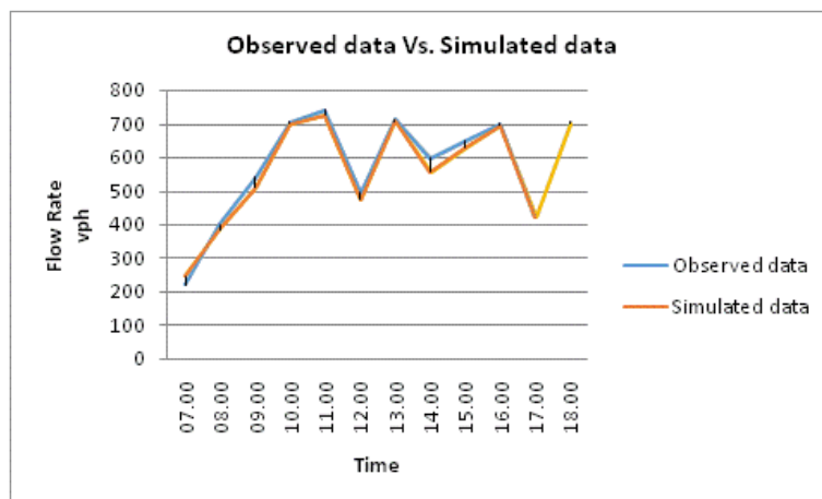
Figure 4.15 : Comparing Simulated data with Field Vehicular Traffic Flow for 12-hour on Saturday June 4 th , 2016 on Link- 1
