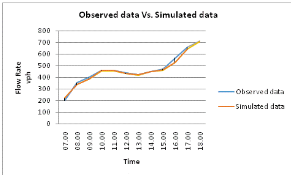
Figure 4.17 : Comparing Simulated data with Field Vehicular Traffic Flow for 12-hour on Wednesday June 8 th , 2016 in Link- 1
