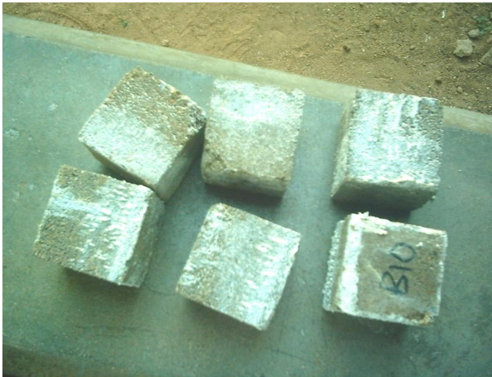
Plate VIII: Mortar cubes suffered from efflorescence as at the 56 th day of curing.
