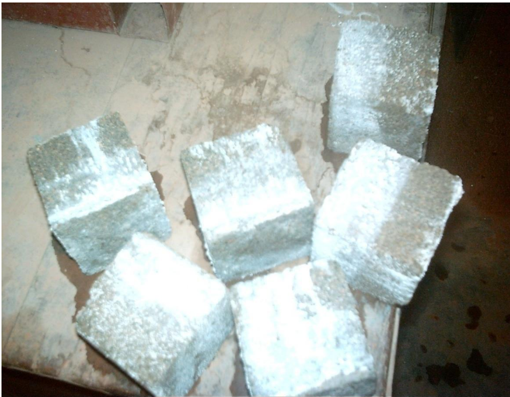
Plate IX: Mortar cubes suffered from efflorescence as at the 90 th day of curing.
