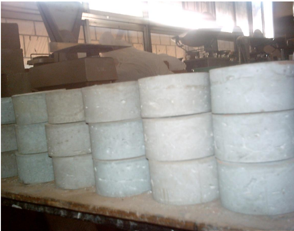
Plate VI: Hardened cement paste specimens for setting time test.
