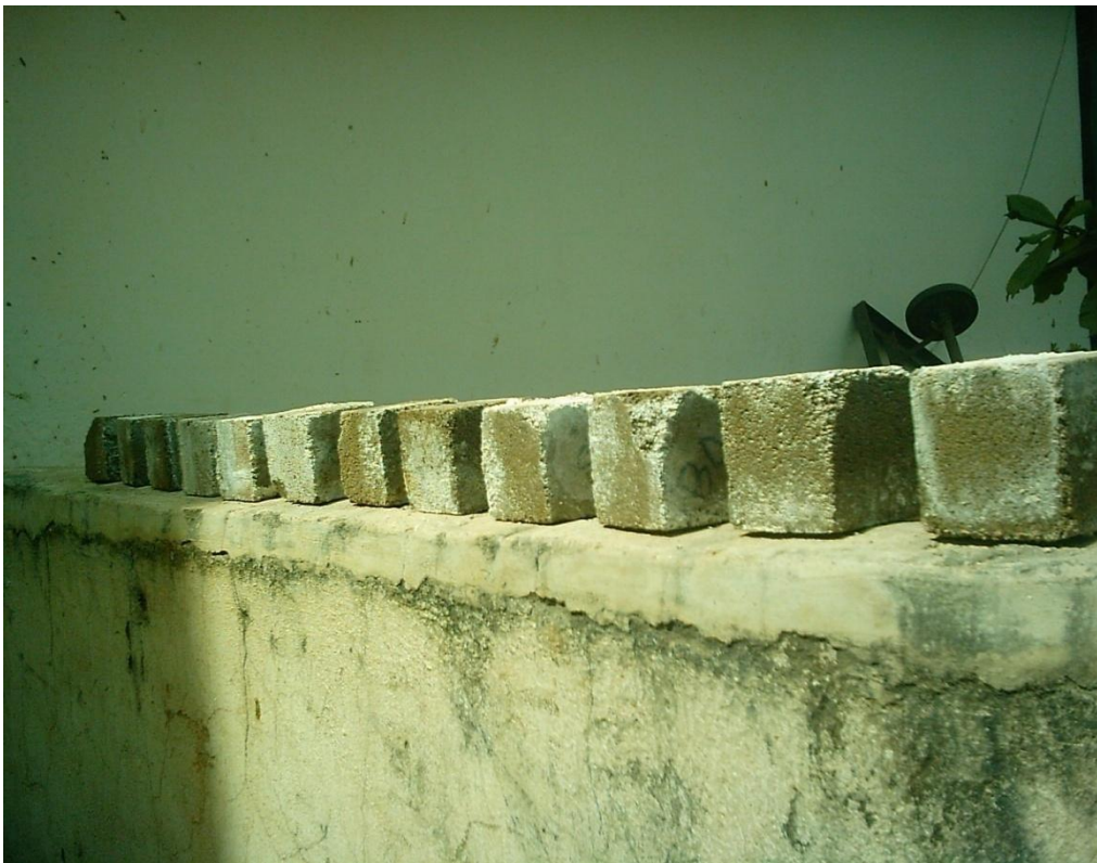
Plate VII: Mortar cubes undergoing drying under the sun for 2 hours
