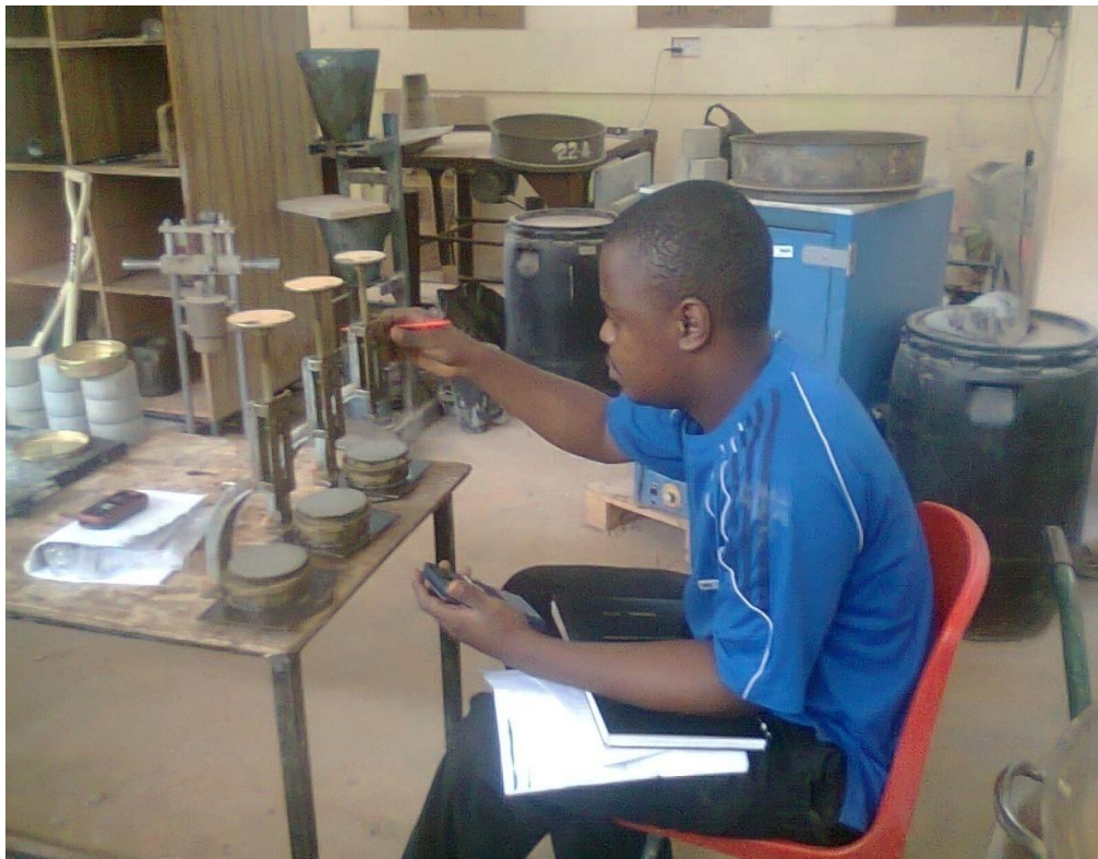
Plate V: Setting time test for control and blended cement paste.
