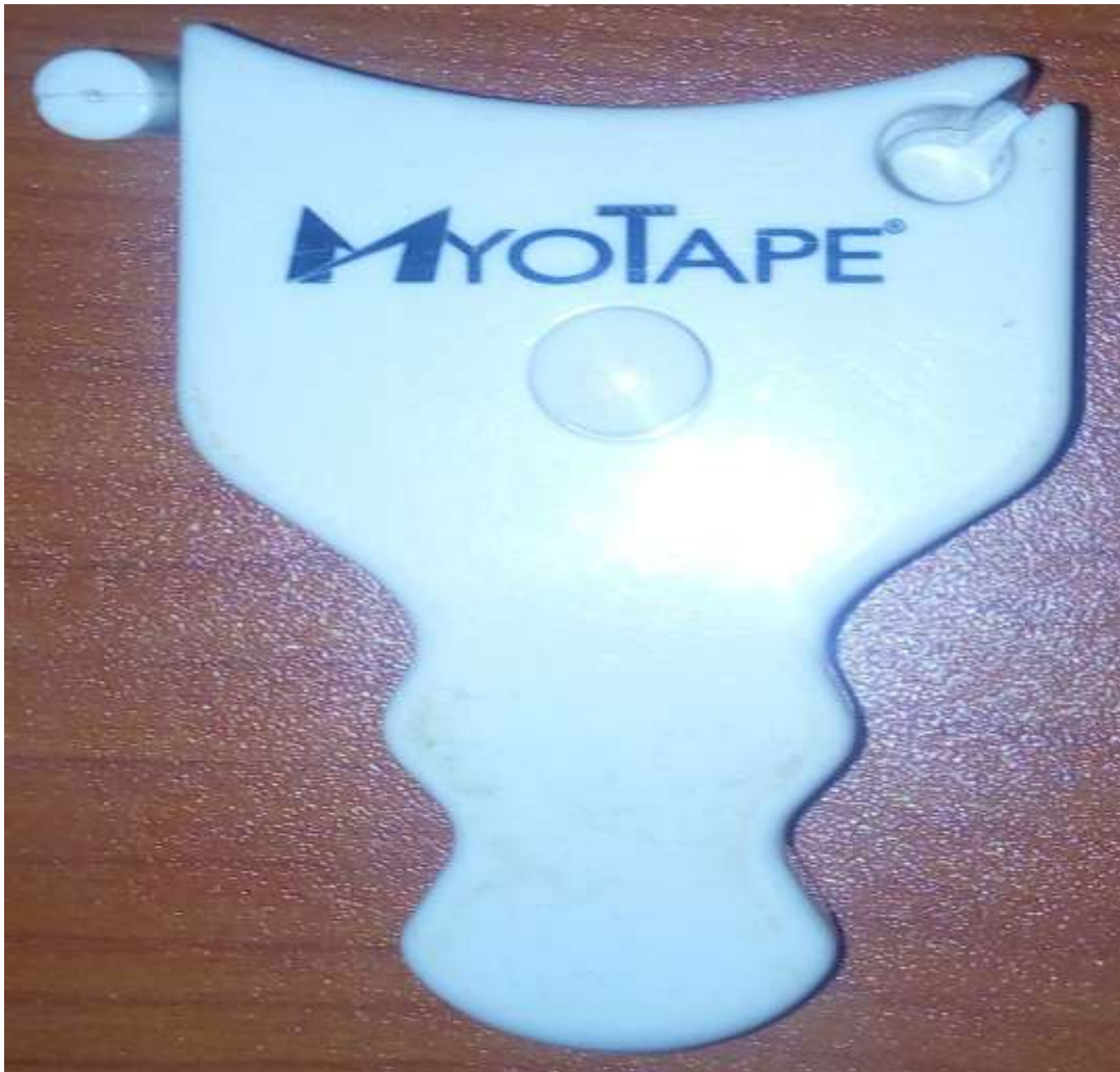
Plate IV: Non-elastic measuring tape (Myotape; AccuFitness, Greenwood Village, Co) for circumferences measurement in cm
