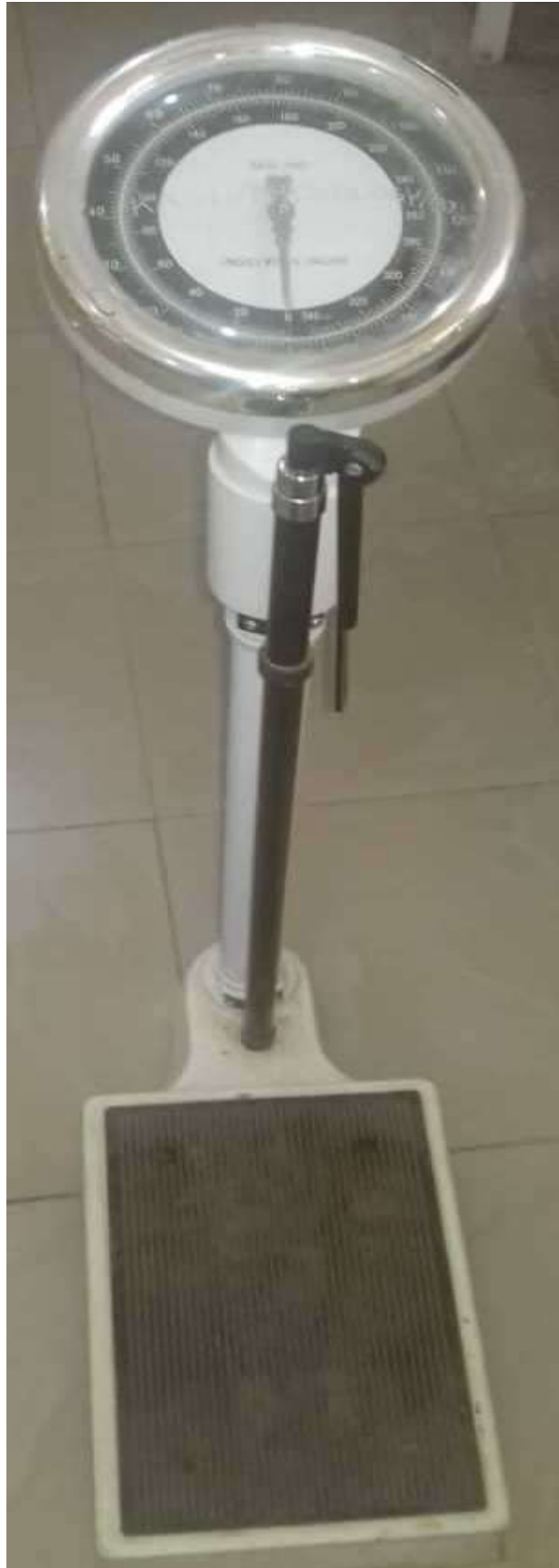
Plate I: Weighing balance with anthropometer (Angel, 150 MA; Istanbul/Turkey) for weight (kg) and height (cm) measurement
