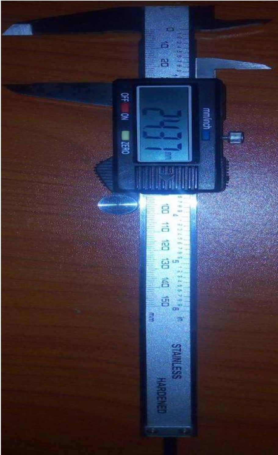
Plate III: Digital sliding caliper (Holtain Ltd, United Kingdom) for measuring Bipicondylar breadth in mm.
