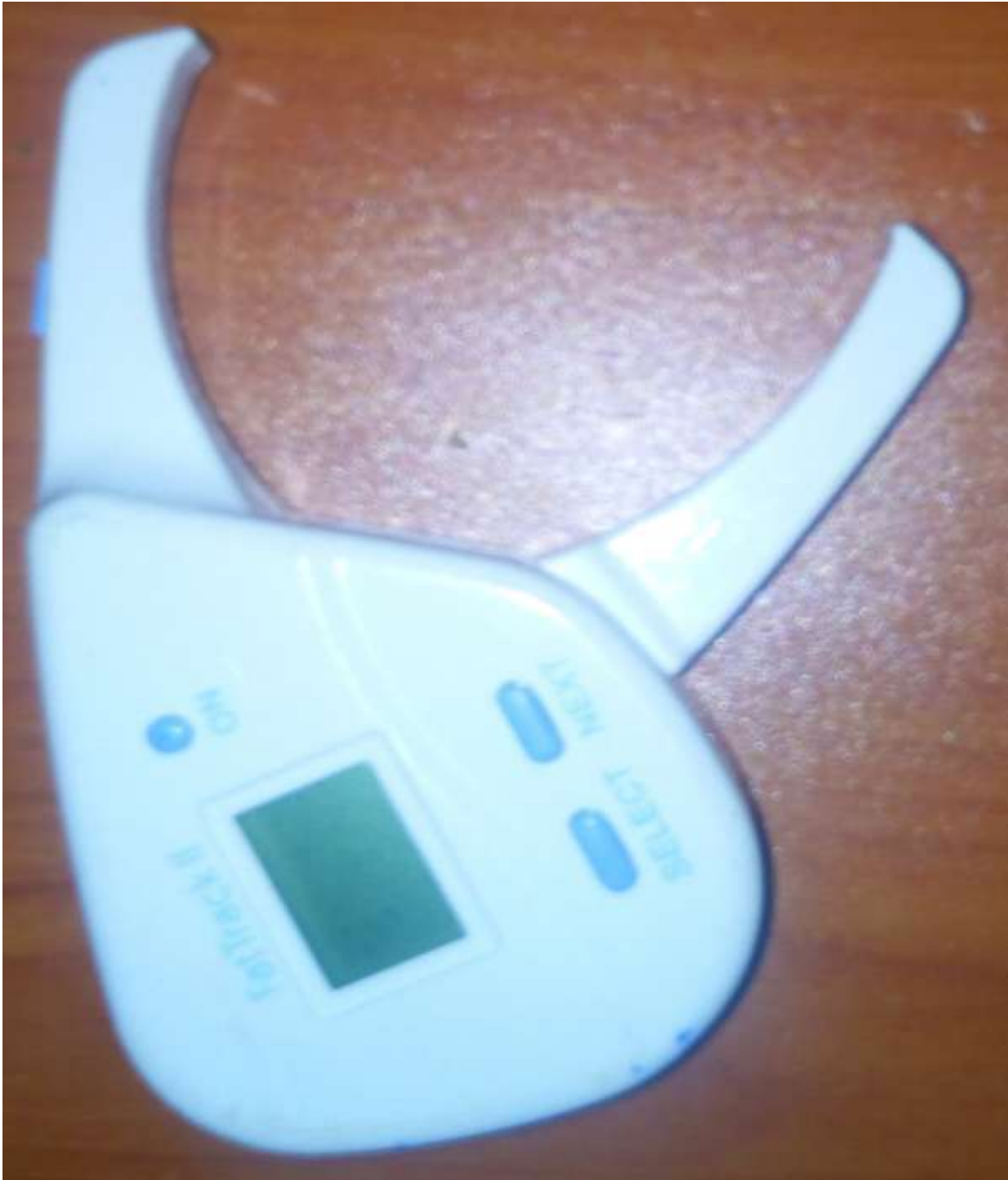
Plate II: Digital body fat caliper (Super Accurate Digital measurement; AccuFitness, Greenwood Village, CO) for skinfolds measurement in mm
