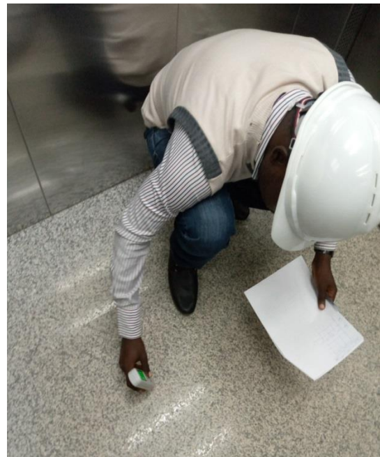
Vibration measurement in standard lift car floor
