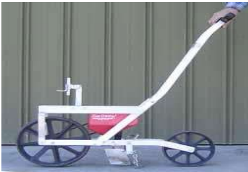
Plate 2.4: Single-row precision planter (Murray et al. , 2006)
