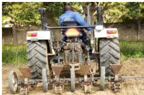
Plate 4.1 Developed Planter Mounted on the Tractor during planting operation
