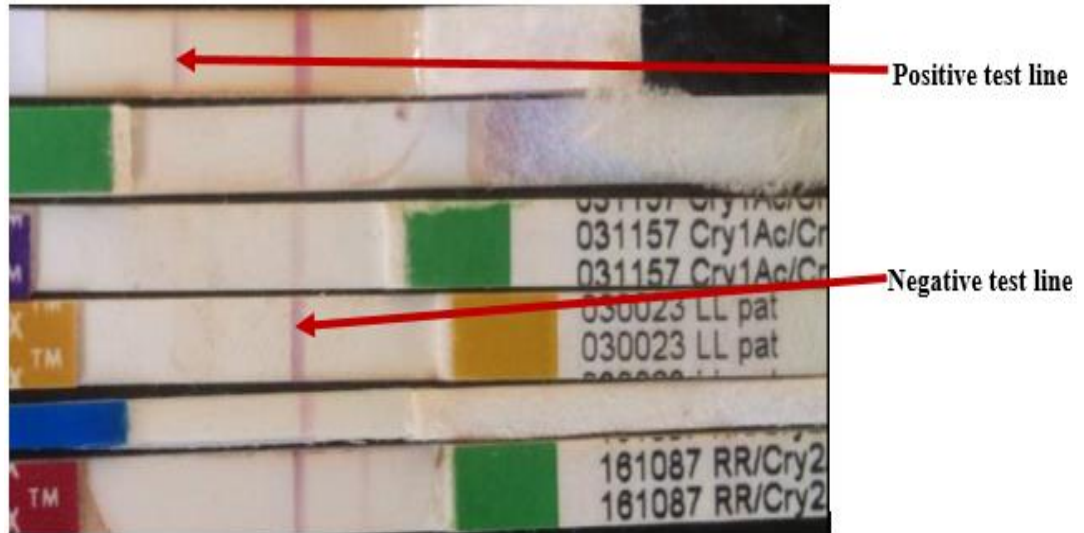
Plate III: Flow strips for CryIAb gene showing positive results for maruca resistant transgenic cowpea and negative for the non-transgenic cowpea line.
