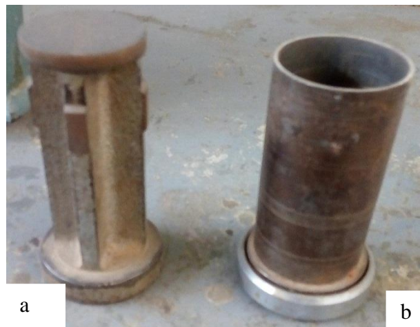
Plate 5: a. Strip for removing cylindrical moulded sample from the mould b. Mould for producing cylindrical moulded sand sample
