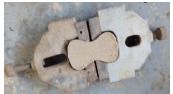
Plate 4: Picture of a gripping device for holding a tensile moulded sample to the universal sand strength testing machine.
