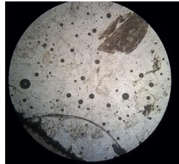
Plate XI: Photomicrograph of Lokoja Sandstone at Filele section making up unit (F/01) of MQ-monocrystalline quartz; PQ-polycrystalline quartz MF –microcline feldspar PF-plagioclase feldspar.
