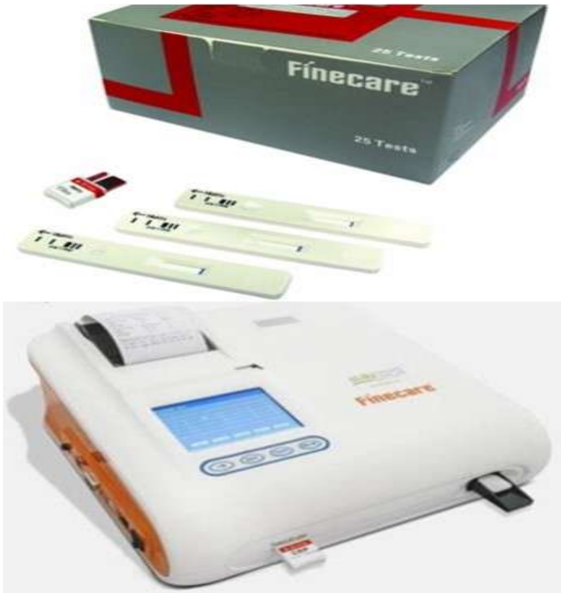
Plate I: The Finecare TM fluorescence immunoassay (FIA) meter, cartridges and ID chip
