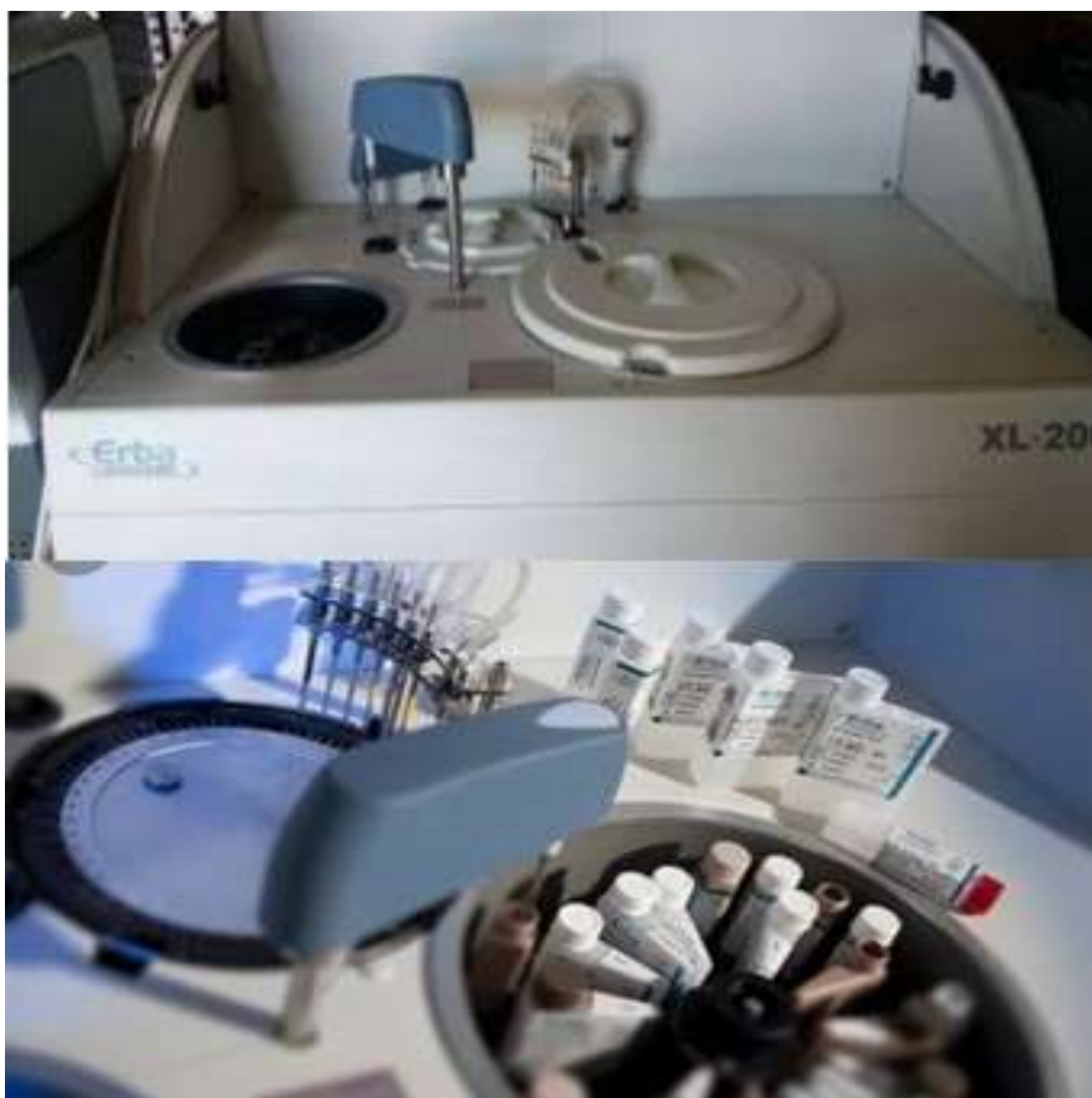
Plate II: The Automated Erba® Mannheim XL-200 Full-Auto Chemistry Analyzer and Reagents for different Analytes
