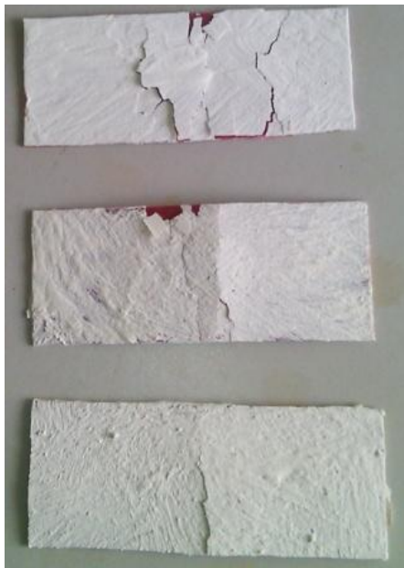
Plate XII: The test panels for the bend test
