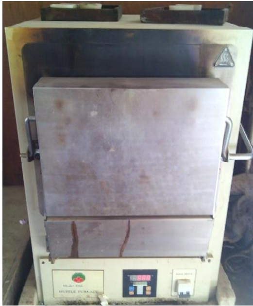
Plate XIII: SXL Muffle furnace and some of the crucibles used for the ash test
