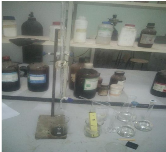
Plate IX: The setup for the determination of the degree of deacetylation
