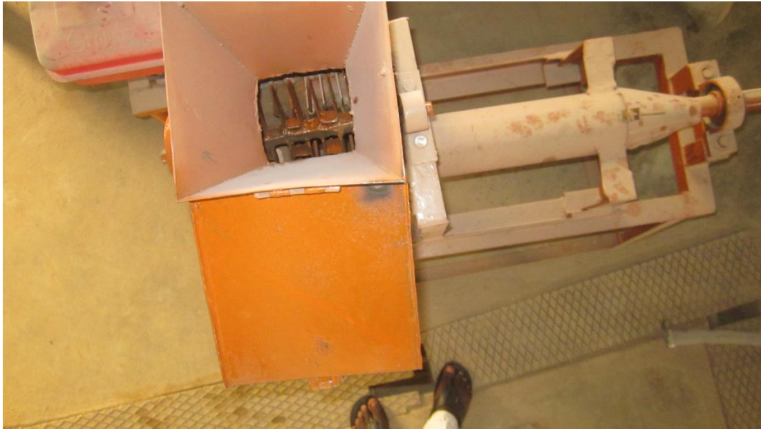
Plate C5: Photograph of the chopping unit showing spikes on shaft
