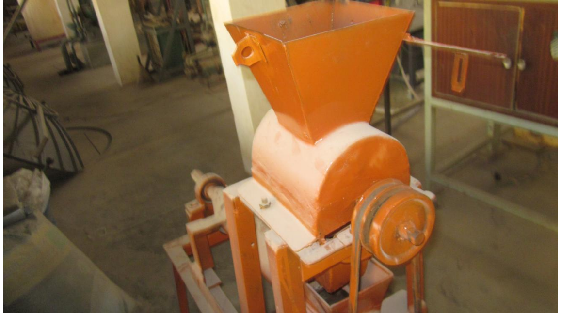
Plate C2: Photograph of the chopping compartment of the extractor
