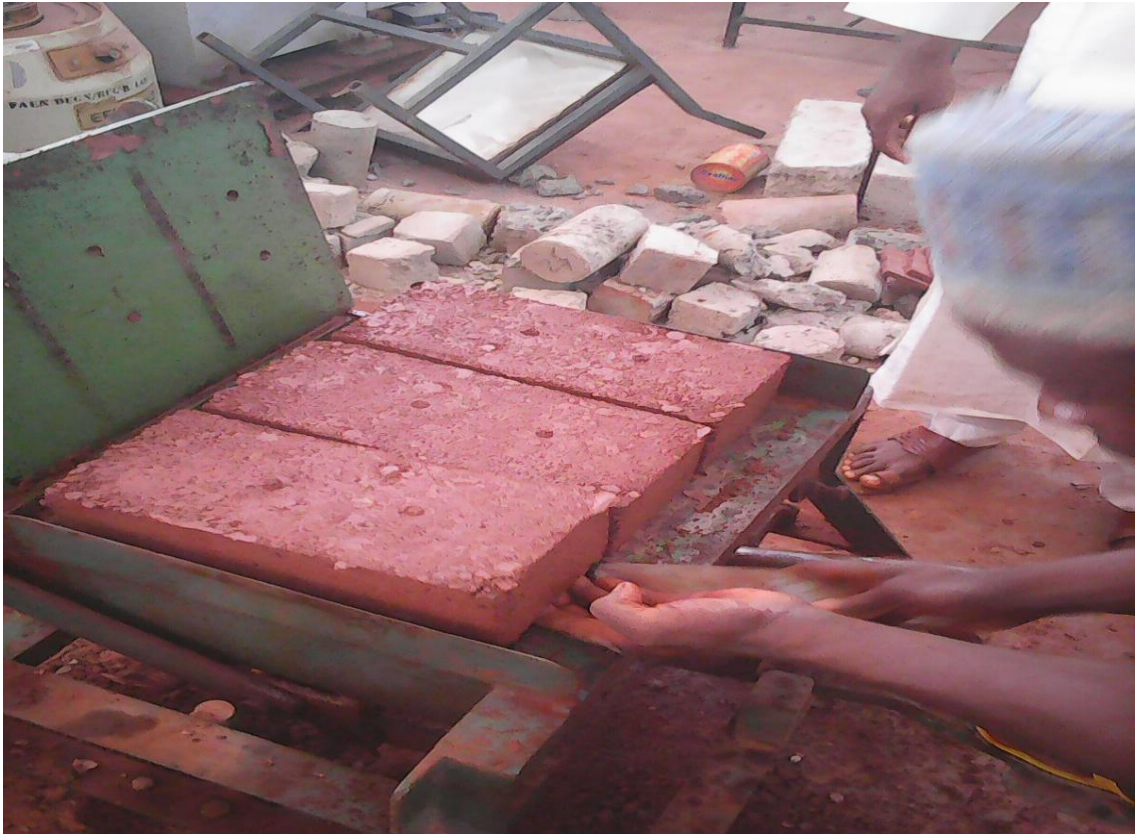
Plate VII De-moulding of Bricks
