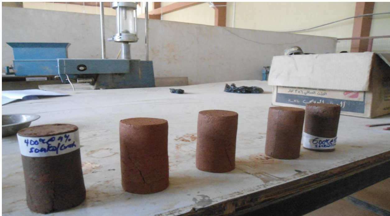
Plate V: Failure pattern of the UCS Specimen
