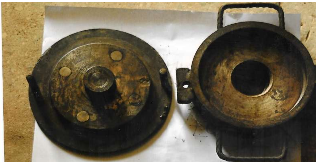
Plate 4.23: Designed and Constructed Mould consisting of the Male and Female Parts used for the Compression Moulding Process of Industrial Oil Seals useful in Bambury Mixers (Two Roll Mills)
