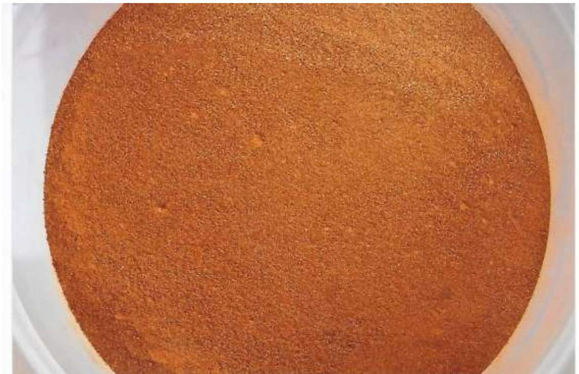
Plate 4.16: Sample of Grounded Coconut Shell Waste and Sieved to 100 \mu\text{m}
