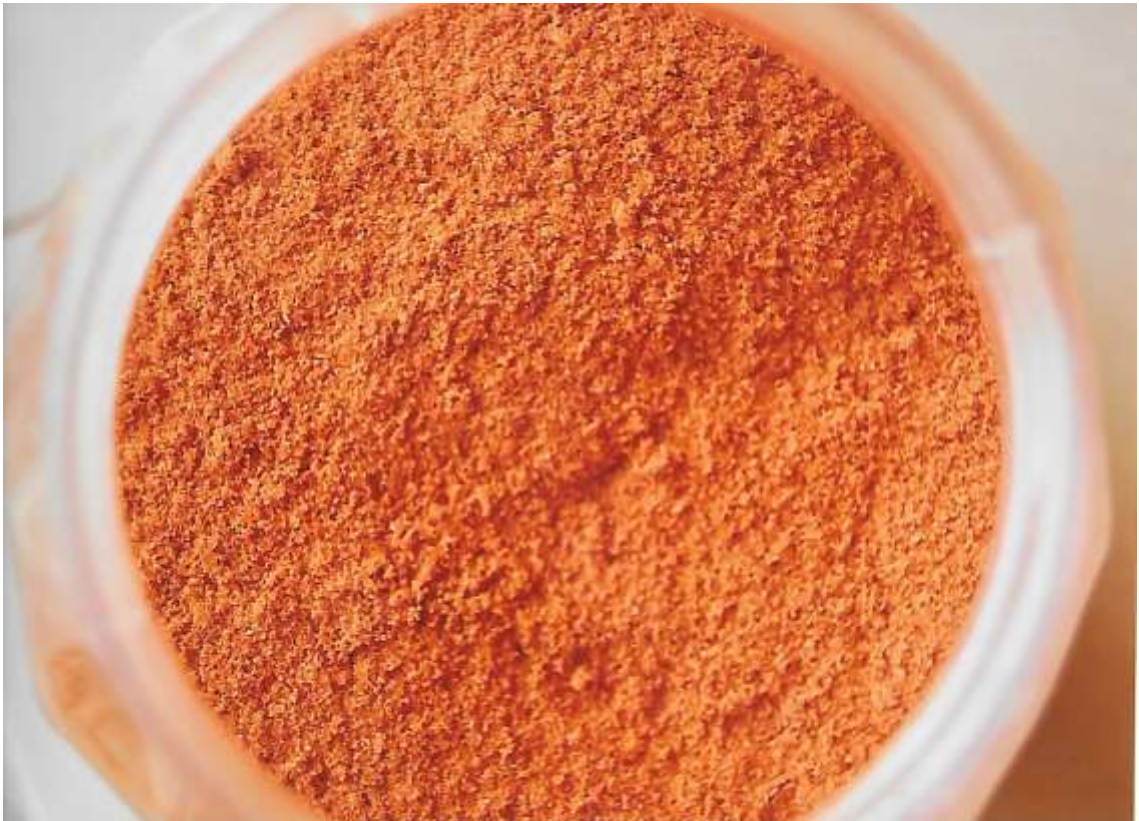
Plate 4.15: Sample of Grounded Coconut Fibre Waste and Sieved to 100 \mu\text{m}
