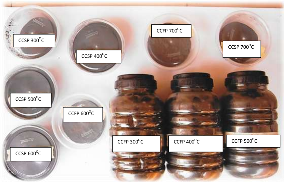
Plate 4.17: Samples of Carbonised Coconut Shell and Fibre Treated at Various Temperatures of 300°C, 400°C, 500°C, 600°C, 700°C and Sieved to 100µm
