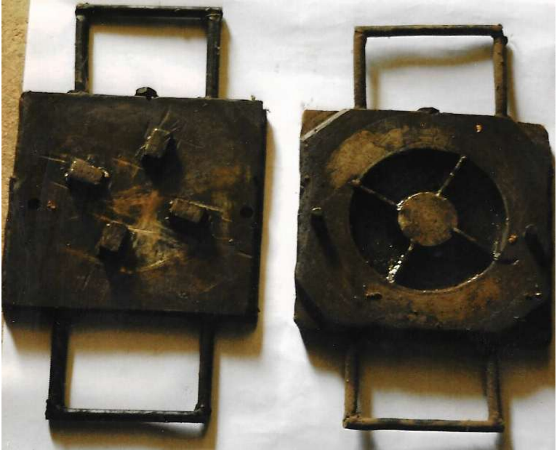
Plate 4.22: Designed and Constructed Mould consisting of the Male and Female Parts used for the Compression Moulding Process of Vibration Dampeners of Motor Cycle Hub
