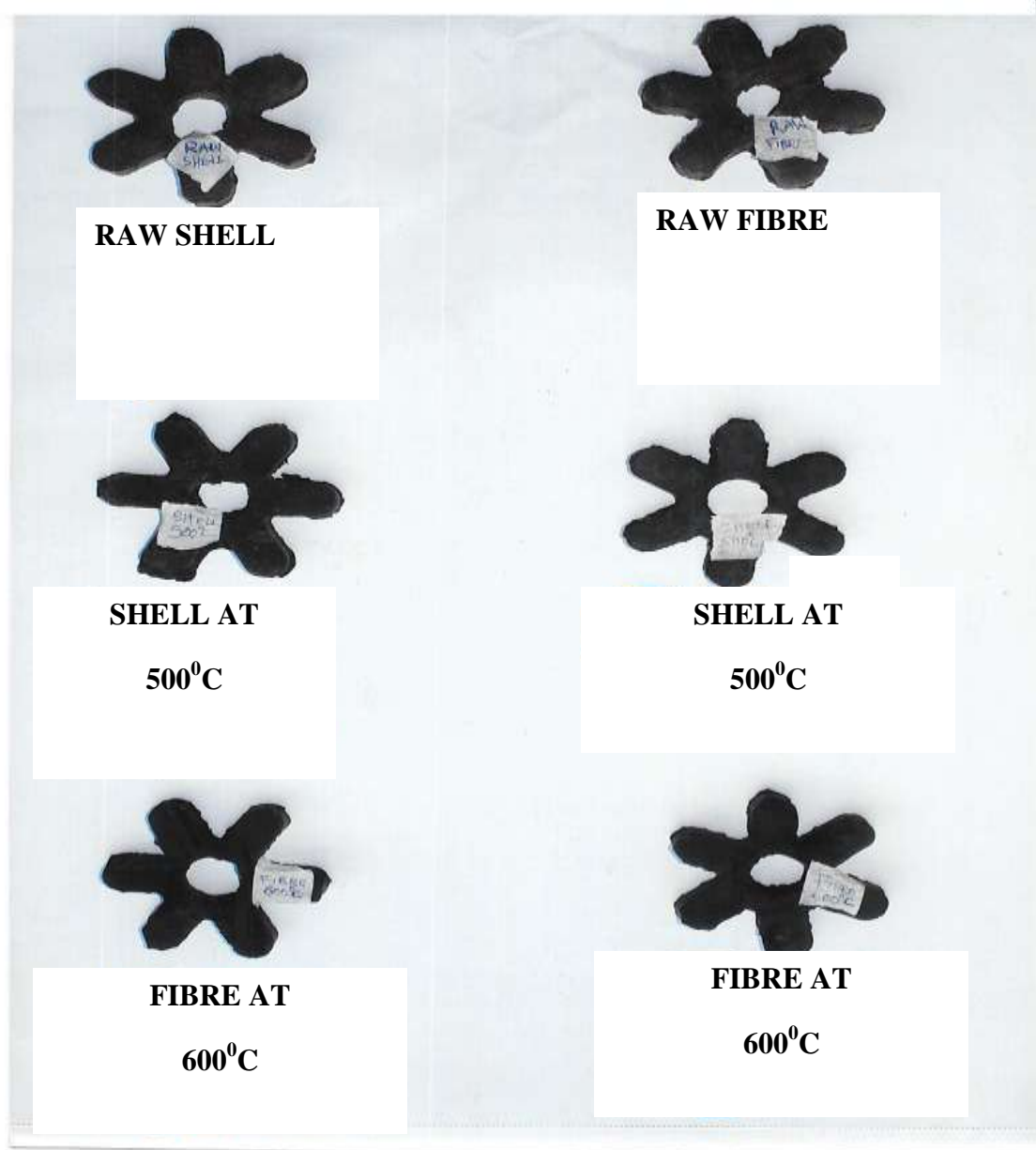
Plate 4.20: Vibration Dampeners for Motor Cycle Hubs from Optimised Formulation of Raw Coconut Shell, Raw Coconut Fibre, Carbonised Shell at 500°C and Carbonised Fibre at 600°C
