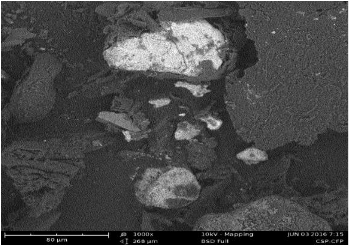
Plate 4.7: SEM Monograph of Composite with Raw Coconut Shell
