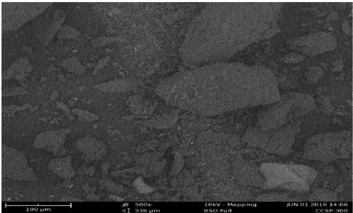
Plate 4.2: SEM Monograph of Composite with Coconut Fibre at 300°C
