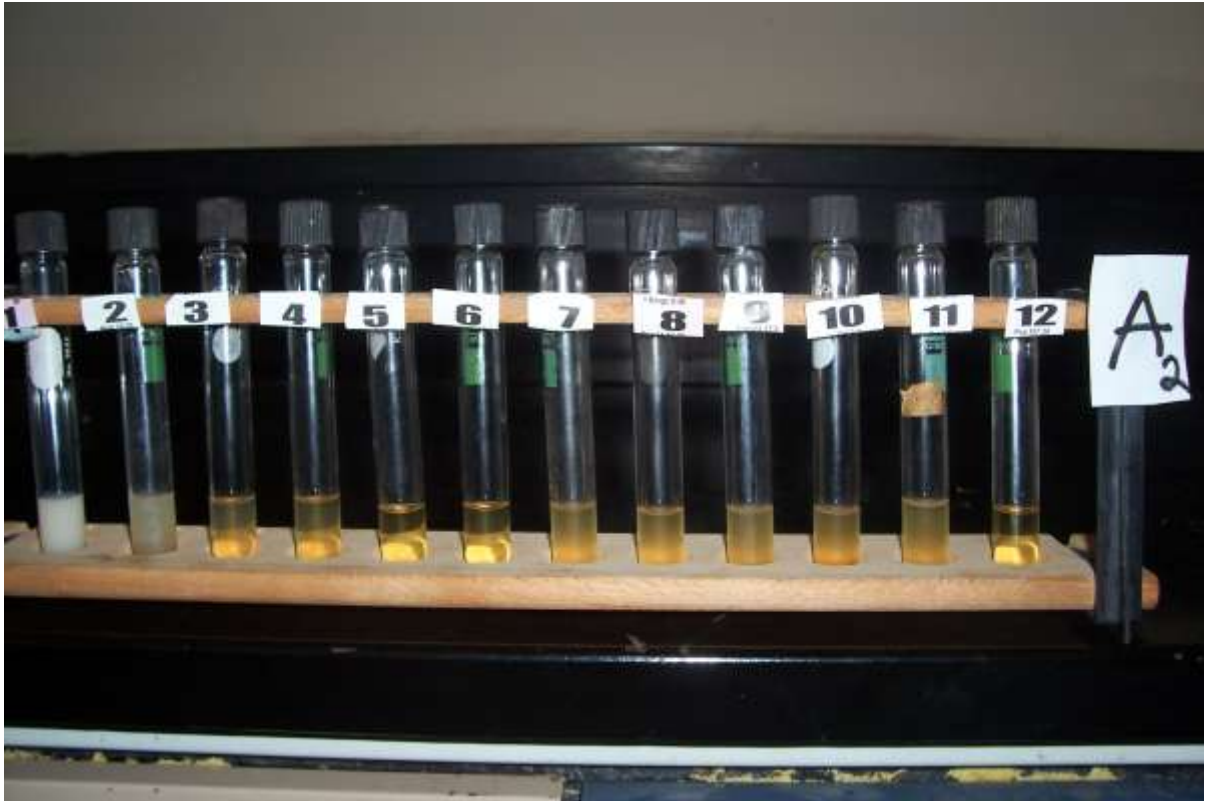
Plate III: MIC determination of carcil ® on E. coli MIC at tube 7 Tube 12 is negative control
