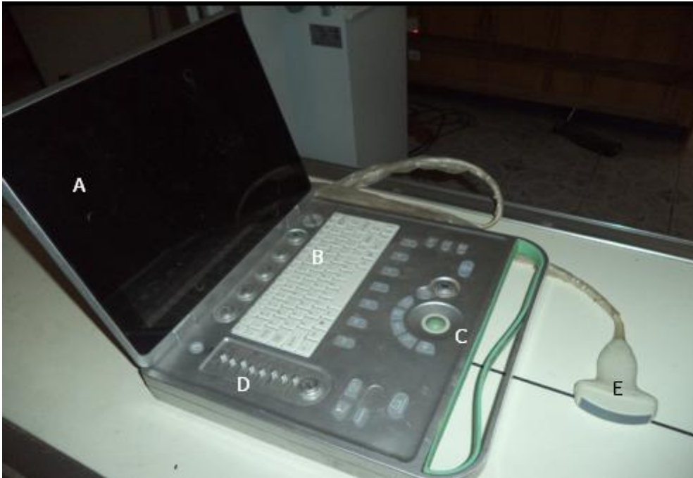
Plate 3.5. B-mode Sonostar C5 ultrasound scanner and a 7.5 MHz curvilinear transducer used for the abdominal ultrasound
