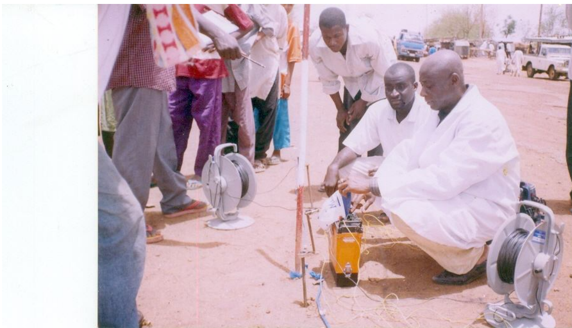
Plate 2: Note line of Electrodes and the Terrameter being operated by the technician from Geophysics Dept. A.B.U, Zaria and Researcher
