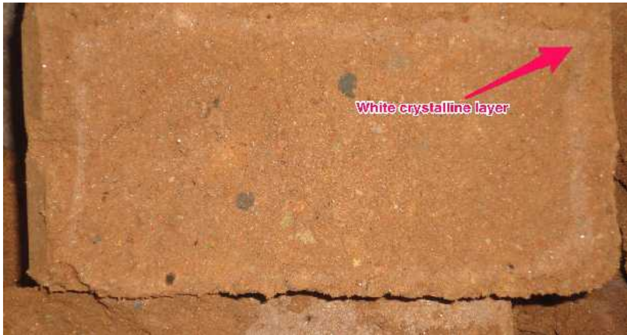
Plate V: White layer deposit within Hydraform block after crushing
