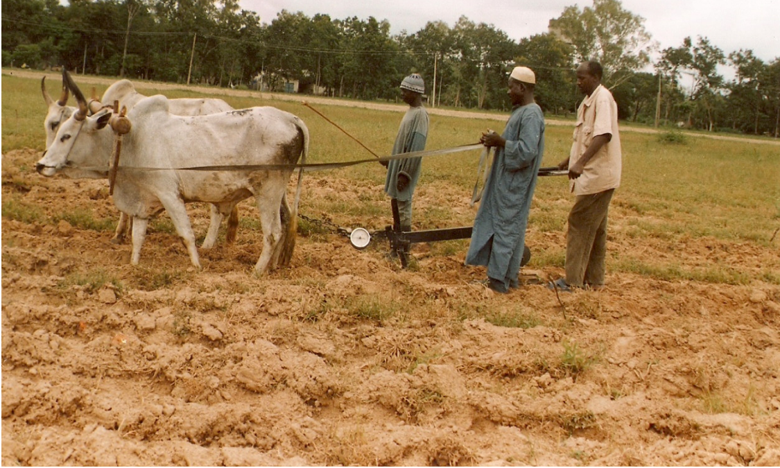
Figure 4.3: Draught animals during operation with dynamometer fitted
