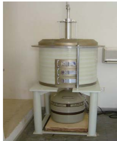
(b) Gamma Ray Spectrometer based on High Purity Germanium Detector
