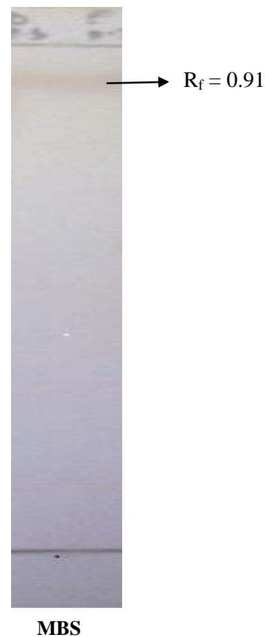
PLATE XI: TLC plate of MBS in diethyl ether: ethyl acetate = 19:1 as sprayed with sulphuric acid.
