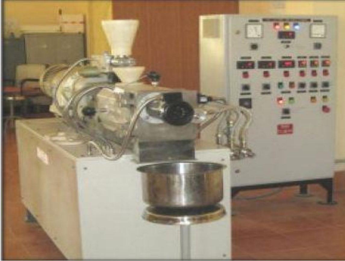
Plate 2.2: Single screw extruder used for preparation of Extruded products (Beladhadi et al. , 2015).
