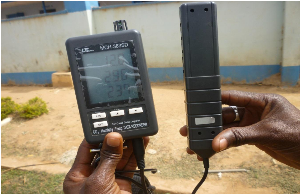
Plate I: The CO 2 / Humidity/ Temperature Data Recorder and the CO 2 Sensor
