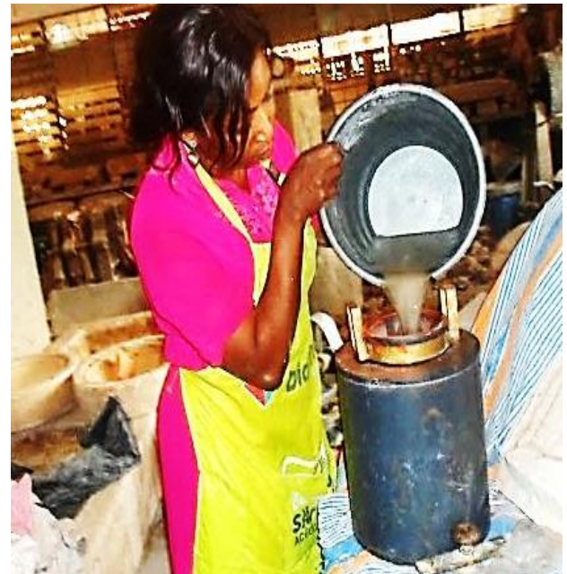
Plate XXXVI: Pouring of Mixed Glaze in Ball Mill Source: Research Photograph, Tser, (2017).
