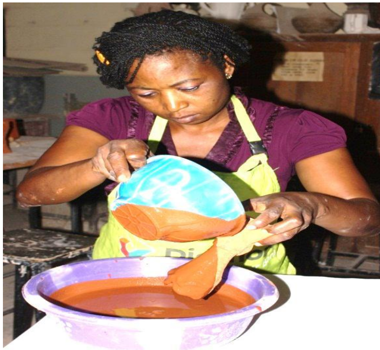
Plate XL: Pouring Method Source: Studio Research, Tser, (2017).
