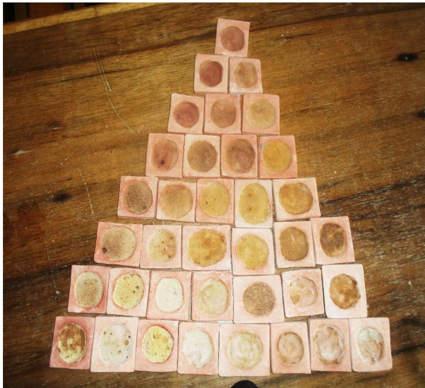
Plate XIII: Tri-axial Blend Test at 900 0 C Fired Source: ResearchPhotograph,Tser, (2017).
