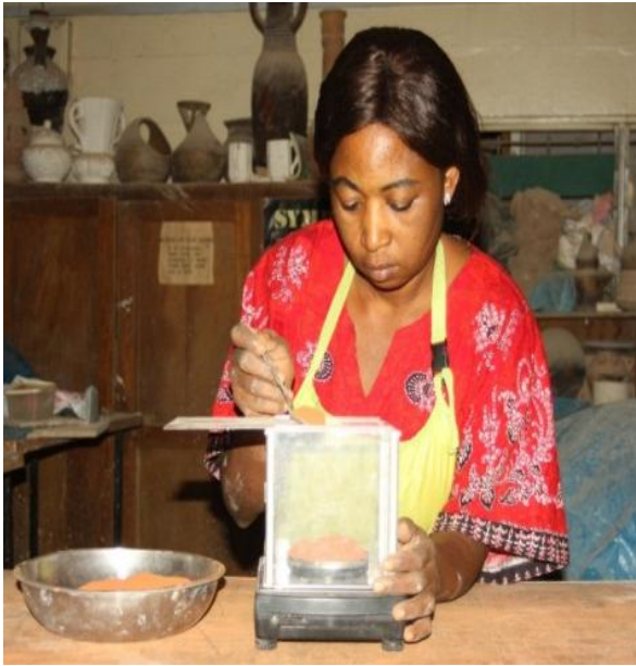
Plate XXXIII: Measuring of Dogo Red Clay Using Digital Scale Source: Research Photograph, Tser, (2017).
