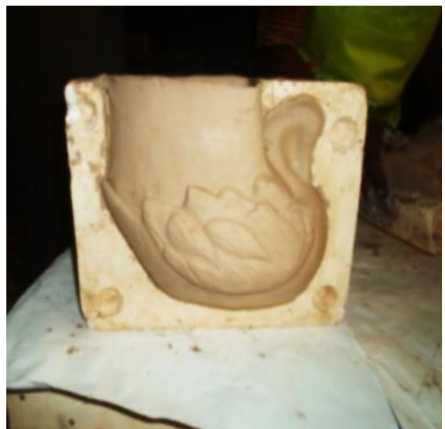
Plate XXIV: Cast Work in the Mould Source: Research Photograph, Tser, (2017).
