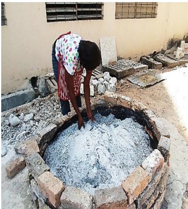
Plate IX: Burning Process of Groundnut Shells Source Research Photograph, Tser (2017)
