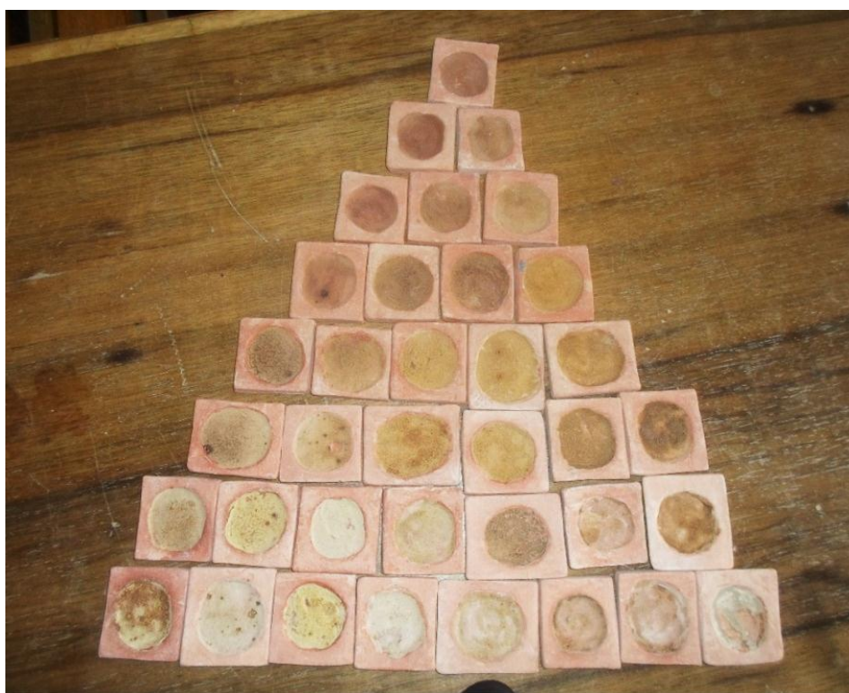
Plate XIV: Tri-axial Blend Test fired at 1000°C Fired Source: ResearchPhotograph, Tser, (2017).
