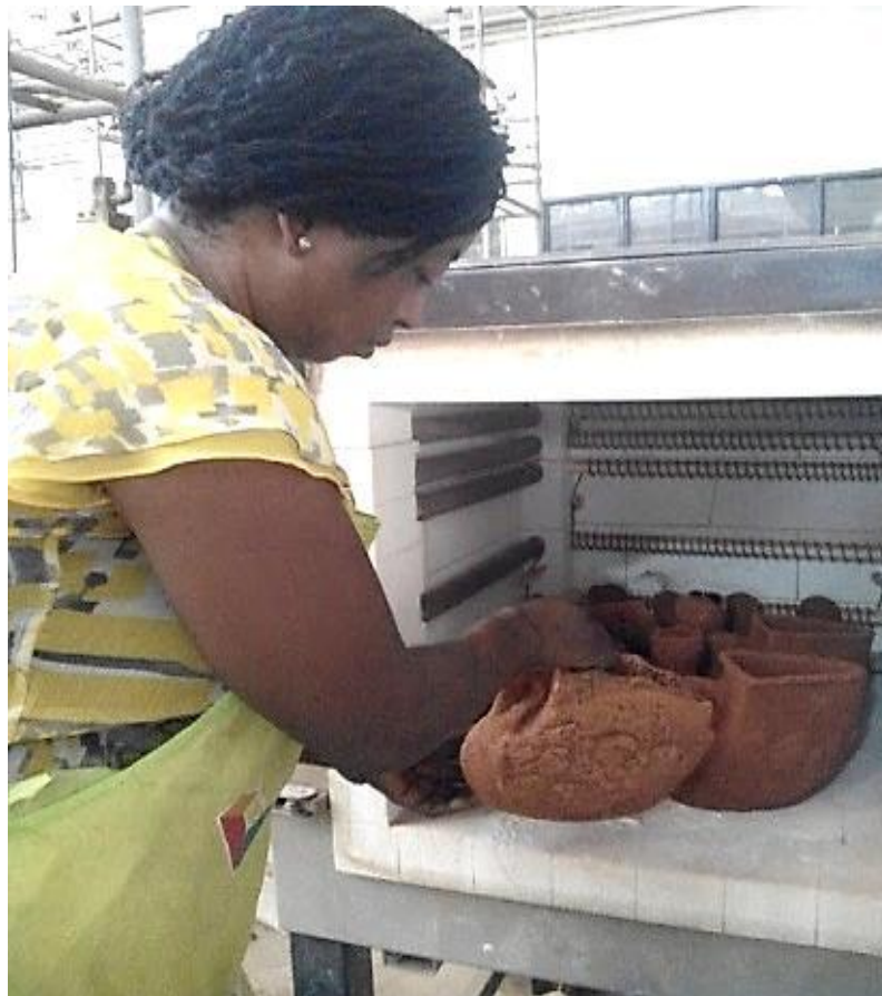
Plate XLIII: Loading Process of Glaze Firing Source: Research Photograph, Tser, (2017).
