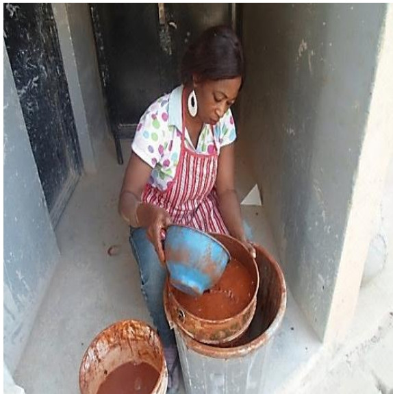
Plate VII: Sieving Process of Dogo Red Clay Source: Research Photograph, Tser (2017)
