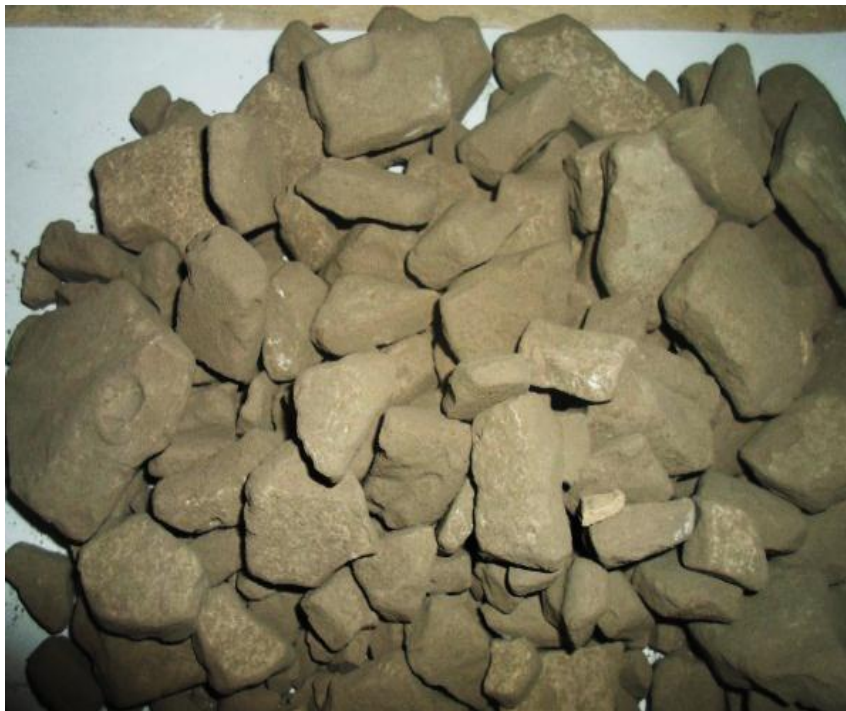
Plate VI: Drying of Groundnut Shells Ash Source: Research Photograph, Tser (2017)
