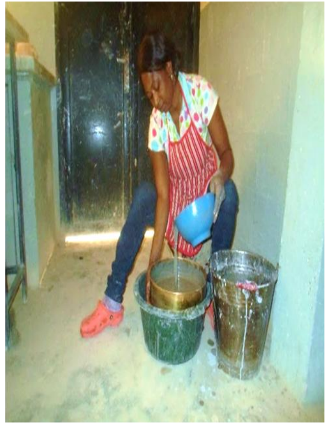
Plate XII: Sieving Process of Locust Bean Wood Ash Source: Research Photograph, Tser (2017)
