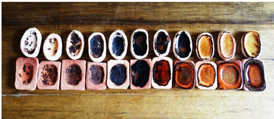
Plate XIX: Line Blend Test 11 member at 1100° C Source: Research Photograph, Tser, (2017).
