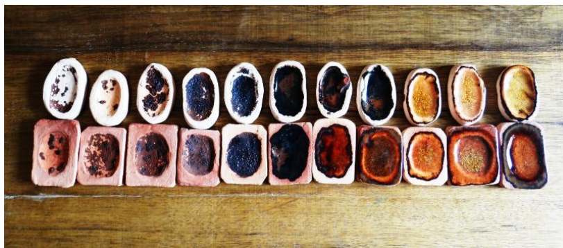
Plate XVII: Line Blend Test 11 member at 900 0 C Source: Research Photograph, Tser, (2017).
