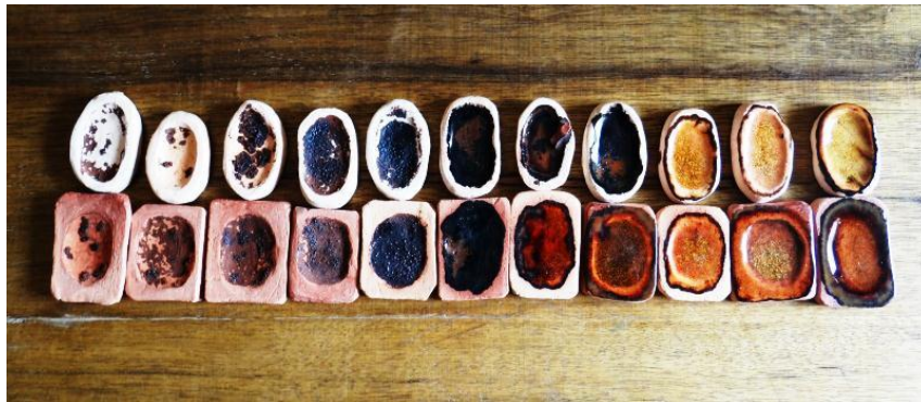
Plate XX: Line Blend Test 11 member at 1160 0 C Source: Research Photograph, Tser, (2017).
