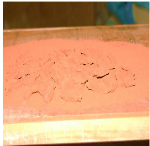
Plate VIII: Drying Process of Dogo Red Clay Source: Research Photograph, Tser (2017)
