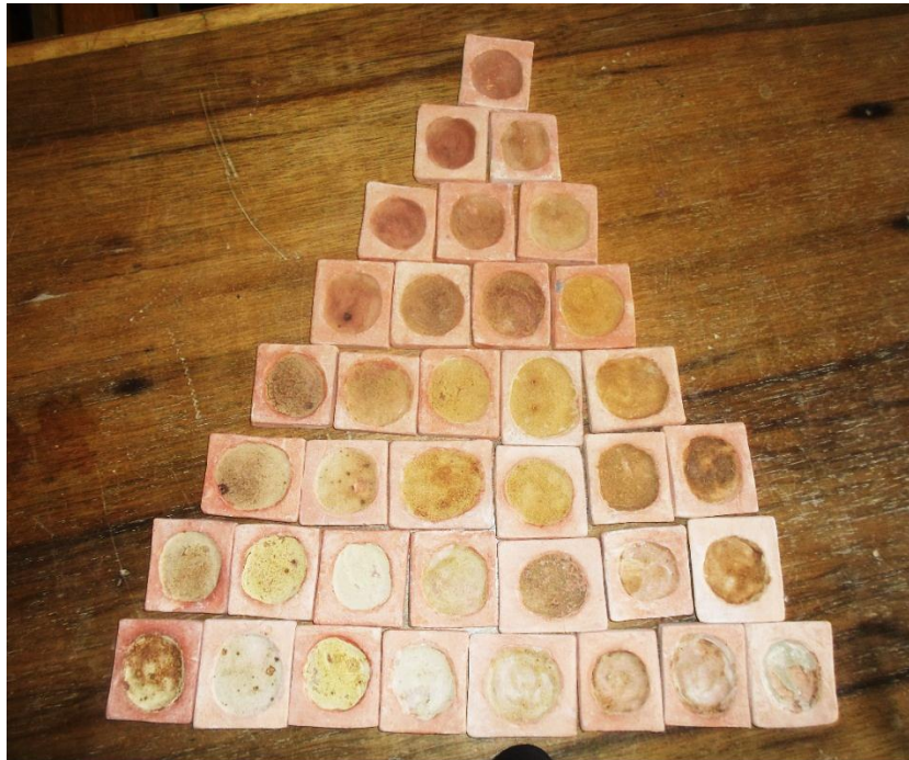
Plate XVI: Tri-axial Blend Test at 1160 0 C Fired Source: Research Photograph, Tser, (2017).
