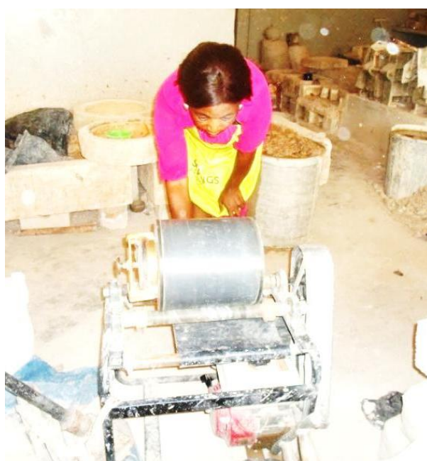
Plate XXXIII: Starting the Ball Mill to mixes the materials for low-temperature glazes Source: Research Photograph, Tser, (2017).
