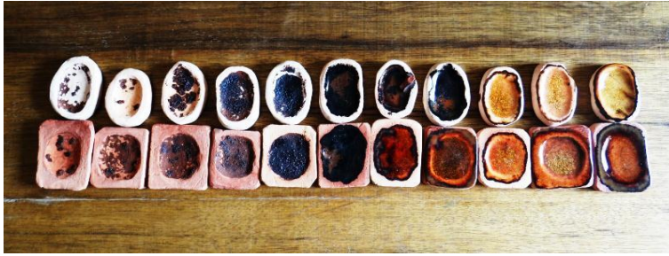
Plate XVIII Line Blend Test 11 member at 1000°C Source: Research Photograph, Tser, (2017)
