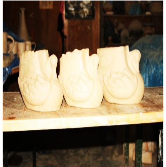
Plate XXX: Leather Hard Cast Work Source: Research Photograph, Tser, (2017).
