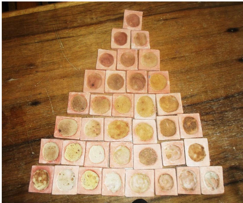
Plate XV: Tri-axial Blend Test at 1100 0 C Fired Source: Research Photograph, Tser, (2017).
