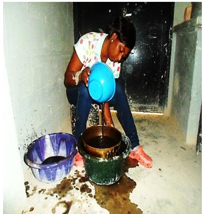
Plate X: Sieving Process of Groundnut Shells Ash Source: Research Photograph, Tser (2017)
