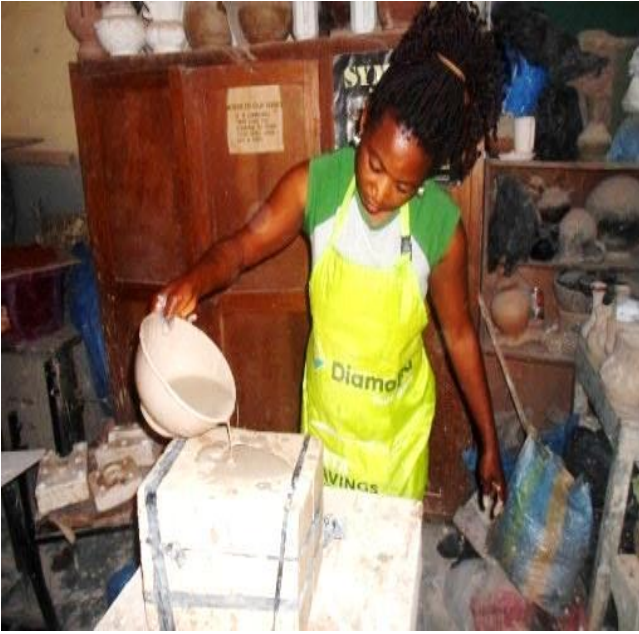
Plate XXI: Pouring Slip inside the Mould Source: Research Photograph, Tser, (2017).
