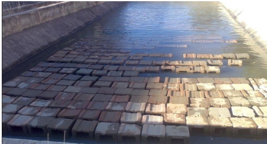
Plate III: Sandcrete hollow blocks soaked in Water
