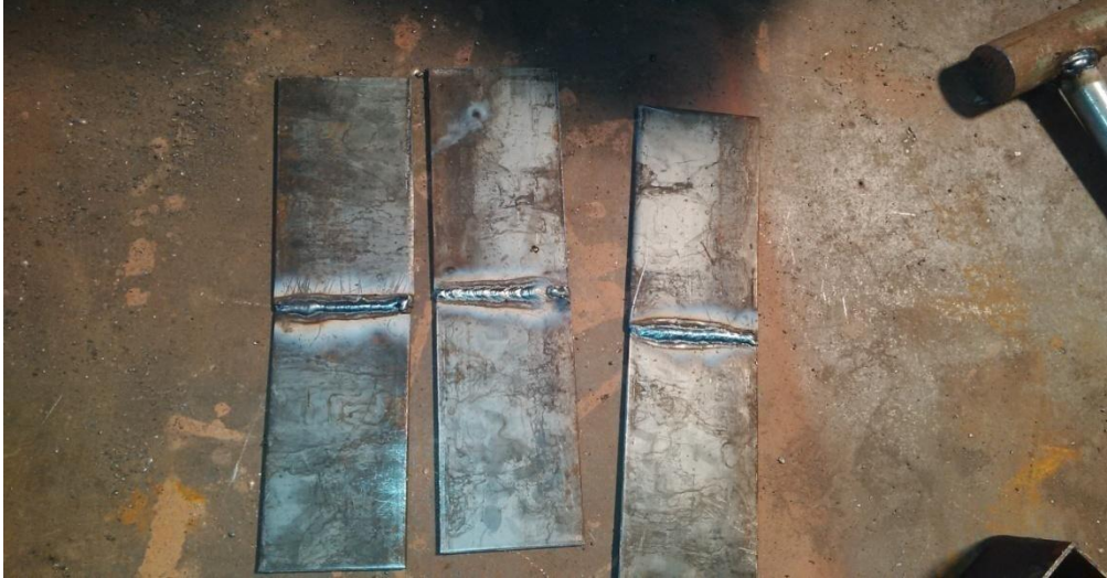
Figure 4.4 Experimental samples of Butt Welded ASTM A36 low Carbon Steel
