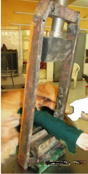
Plate II: Fracture creation. A: Modified Marturano fracture device. B: Experimental dog, C: padded limb of experimental dog placed on limb positioning system, D: Striker
