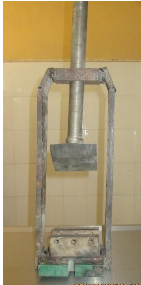
Plate I: Modified Marturano fracture device. A: Shaft, B: Striker, C: Limb positioning system
