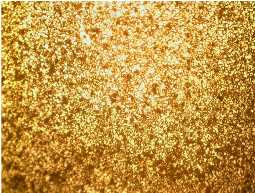
Plate 4.9: Microstructure of medium carbon steel quenched in un-agitated water showing a mixture of martensite and pearlite. Etchant: 2% Nital, Mag. x 200.
