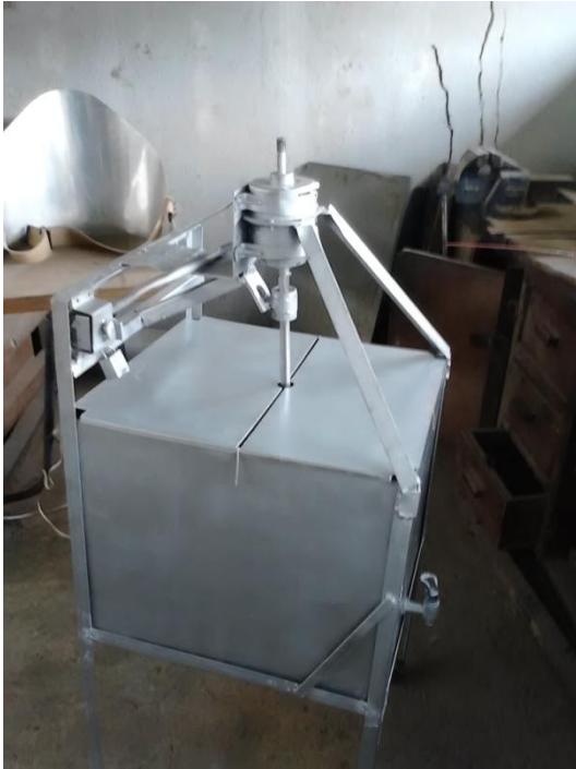
Plate 3.1: Picture of completed quenching bath assembly showing its overall view.
