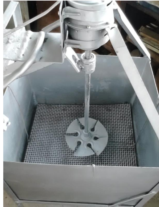
Plate 3.2: Picture of plan view of the quenching bath showing the impeller blades and the suspended wire mesh.
