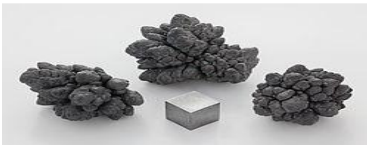
Figure 1.1: Lead Structure (Adopted from Stewart et al. , 2006).
