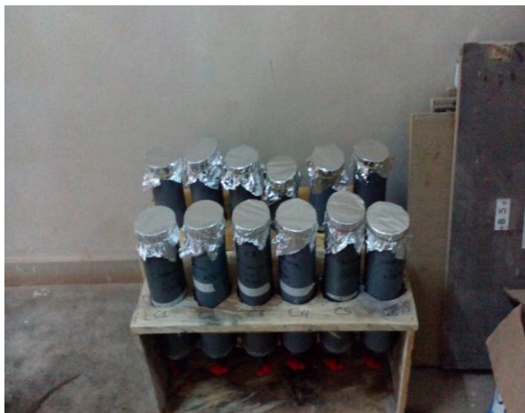
Pictures of sealed Filter Columns before loading
