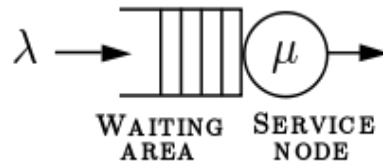
Figure 1.1: A Single Server model (Conceptual model) - the most elementary of queuing model, M/M/1 queuing model, (Sturgul, 2000).
