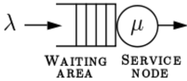
Figure 3.1: A Single Server model (Conceptual model) - the most elementary of queuing model.
