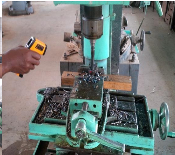
Plate XII: Dry drilling operation of mild steel while measuring the temperature generated with Infrared Thermometer.
