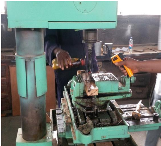
Plate XI: Application of neem seed oil as Cutting fluid in drilling operation of mild steel while measuring the temperature generated with Infrared Thermometer.
