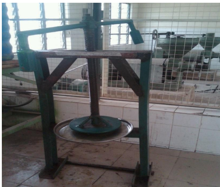
Plate III: Cold Screw Pressing Set up (NARICT, Zaria)
