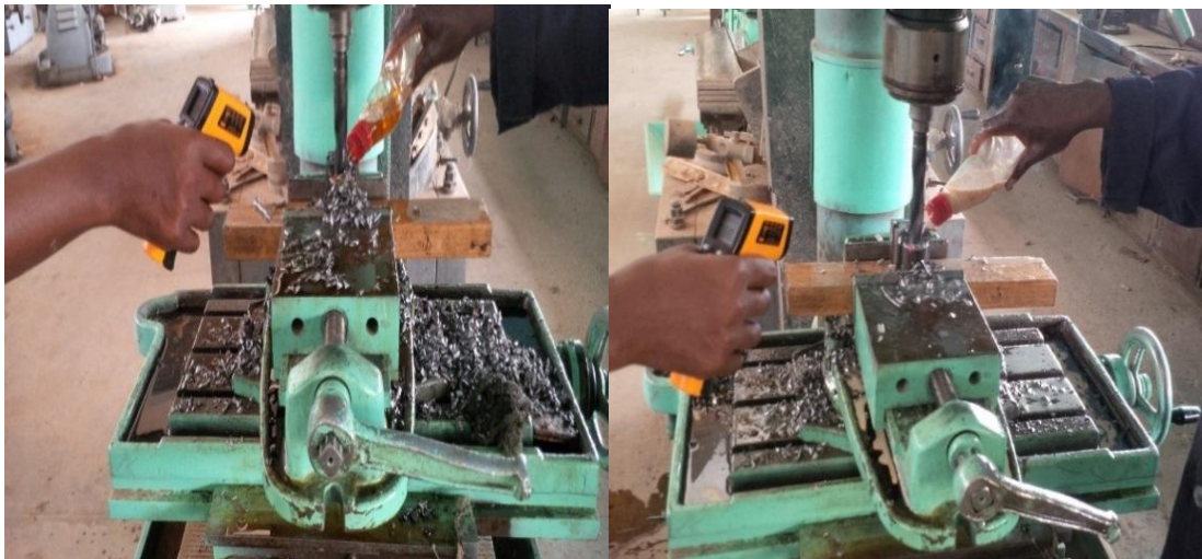
Plate IX: Application of water melon oil as Cutting fluid in drilling operation of mild steel while measuring the temperature generated with Infrared Thermometer. Plate X: Application of soluble oil as Cutting fluid in drilling operation of mild steel while measuring the temperature generated with Infrared Thermometer.
