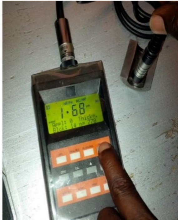
PlateXIV: Measurement of Surface Roughness of drilled part of work piece using Dualscope Fischer device.
