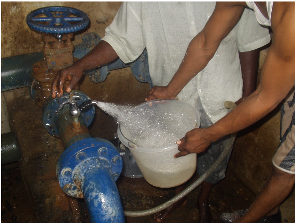
Plate VI: Measuring flow rate at varying pressure
