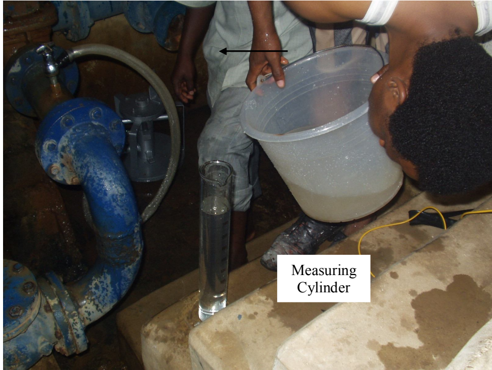
Plate VII: Measuring flow rate at varying pressure
