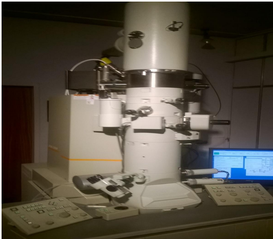
Appendix B2: Photograph of TEM (Jeol, JSM2010)
