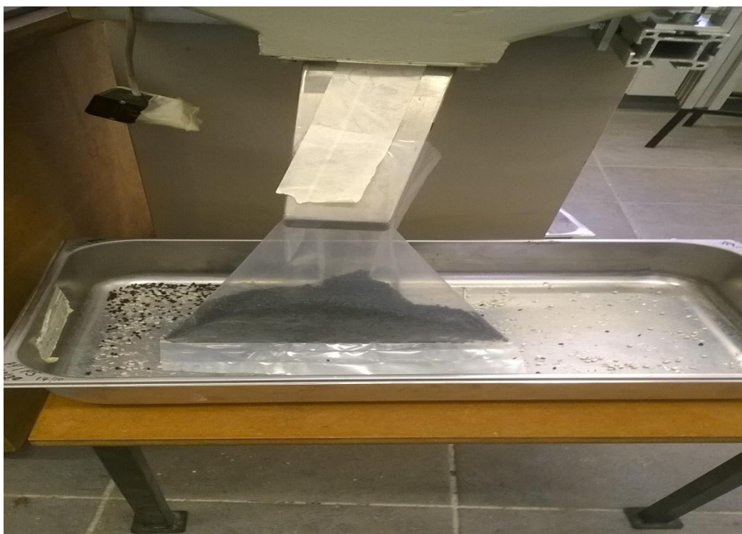
Appendix B8: Photograph of pelletizing of the extrudates
