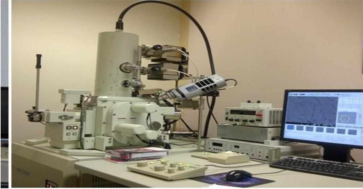
AppendixB12: photograph of JEOL 6480 LV electron microscope
