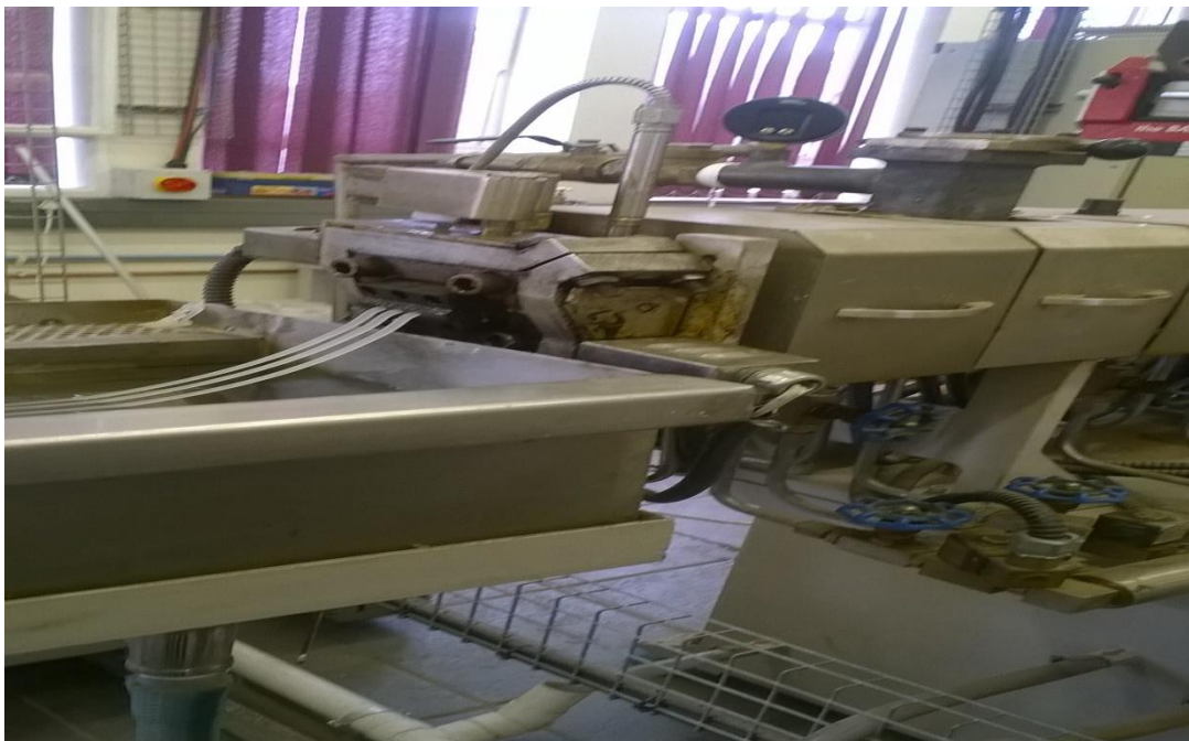
Appendix B7: Photograph of TE-30 Co-rotating screw extruder
