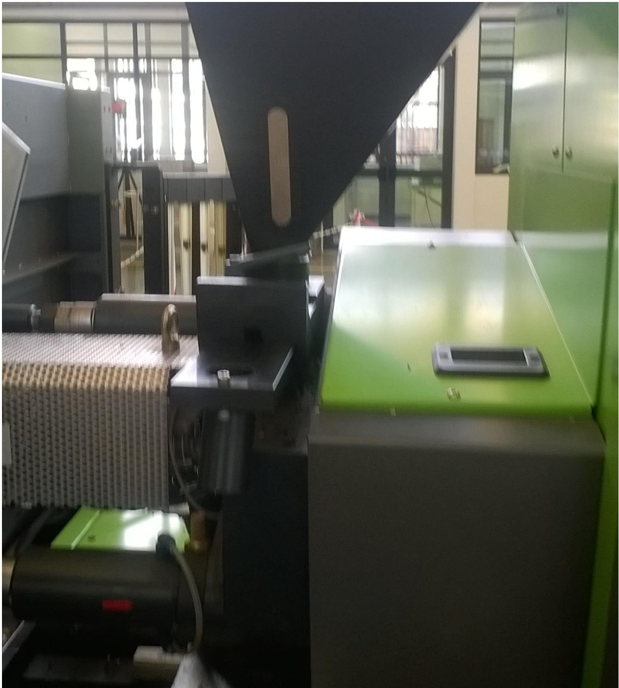
Appendix B9: Photograph of the ENGEL e-mac 50, injection moulding machine
