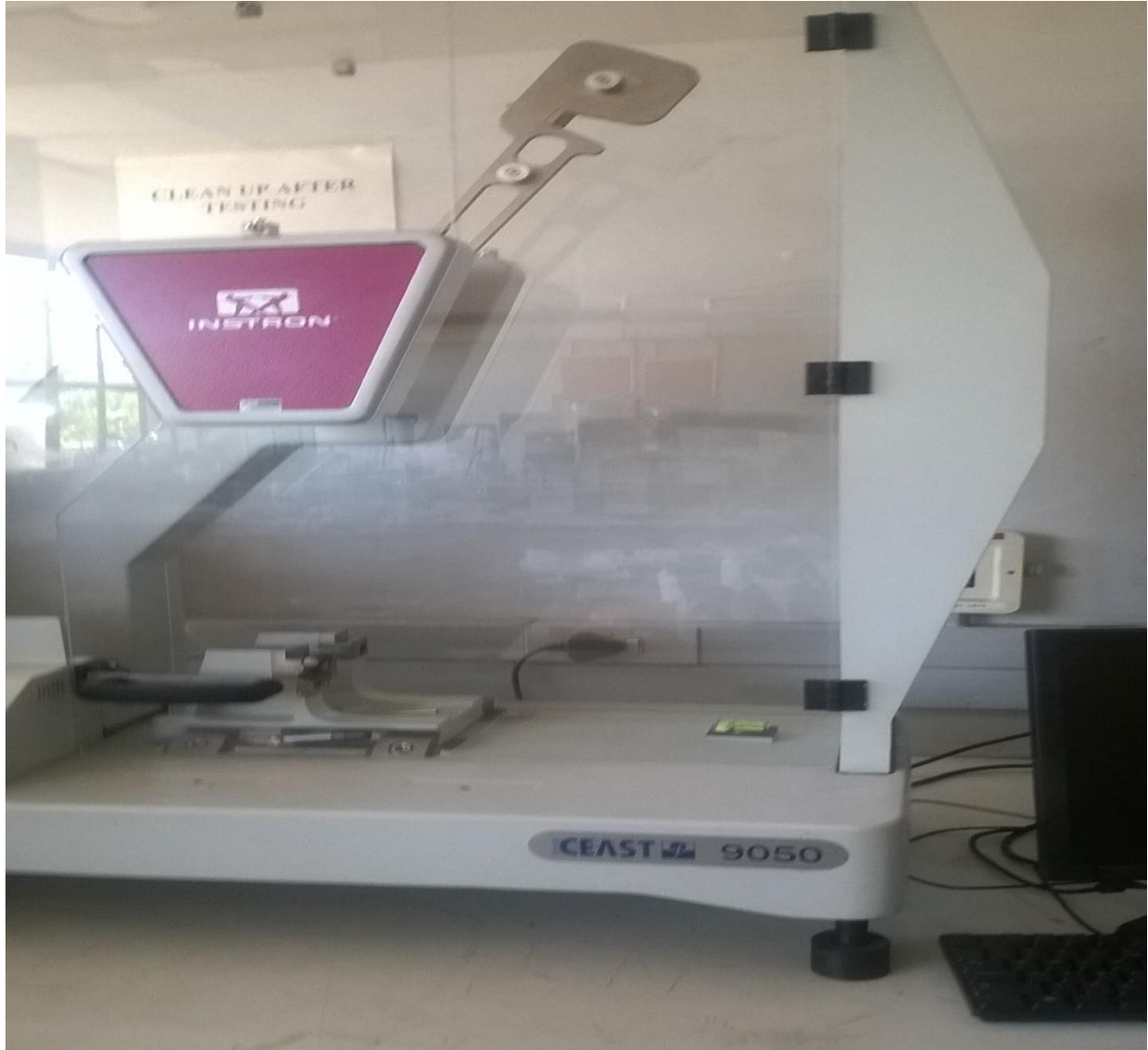
Appendix B11: photograph of Instron impact Energy machine
