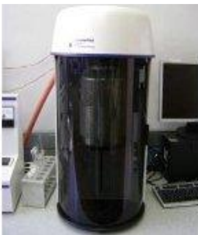
Appendix B3: Photograph of ASAP 2020 Micromeritics surface area analyzer
