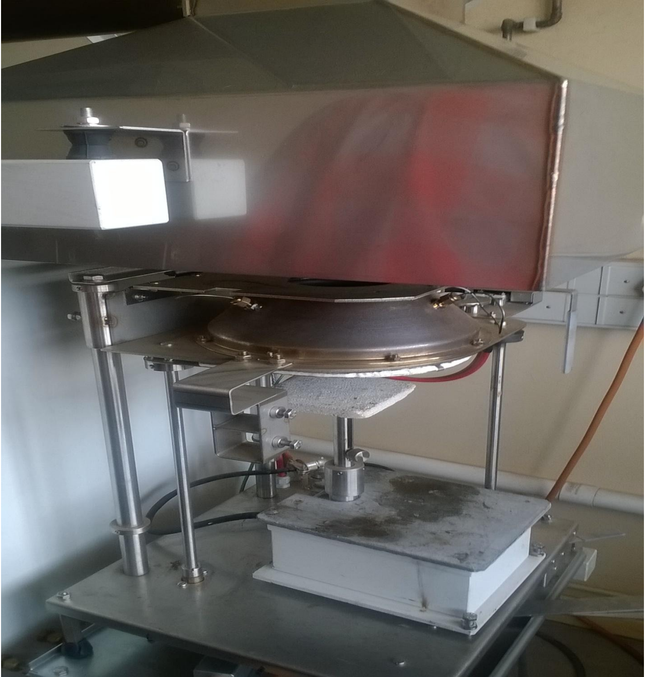
AppendixB14: The cone calorimeter and burning panel inside the calorimeter.
