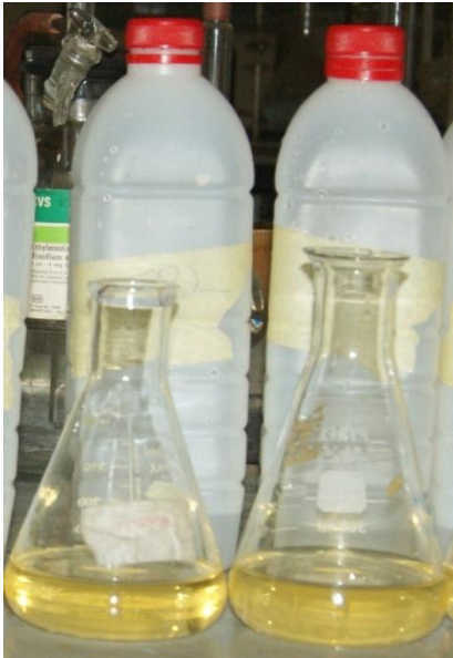
Plate 3.10a: Colour of water samples after adding reagents before titration, in alkalinity determination.
