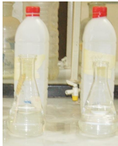
Plate 3.8b: Colour of samples after titrating to the end point (colourless).
