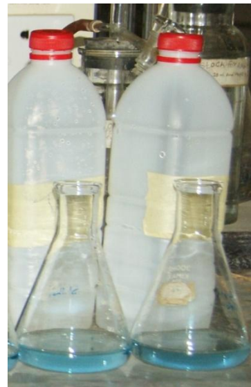
Plate 3.9b: Colour of samples after titrating to the end point (blue colour).
