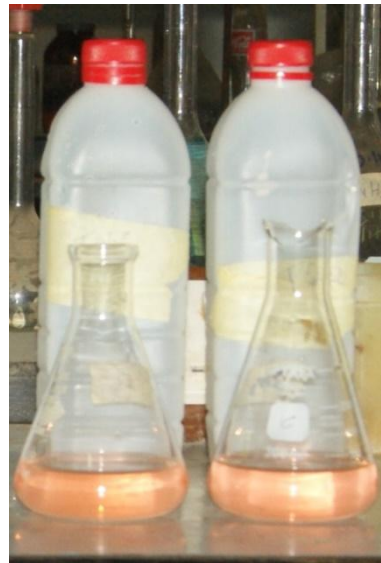
Plate 3.10b: Colour of samples after titrating to the end point (orange colour).
