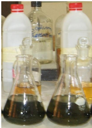
Plate 3.8a: Colour of water samples after adding reagents before titration, in D.O determination.
