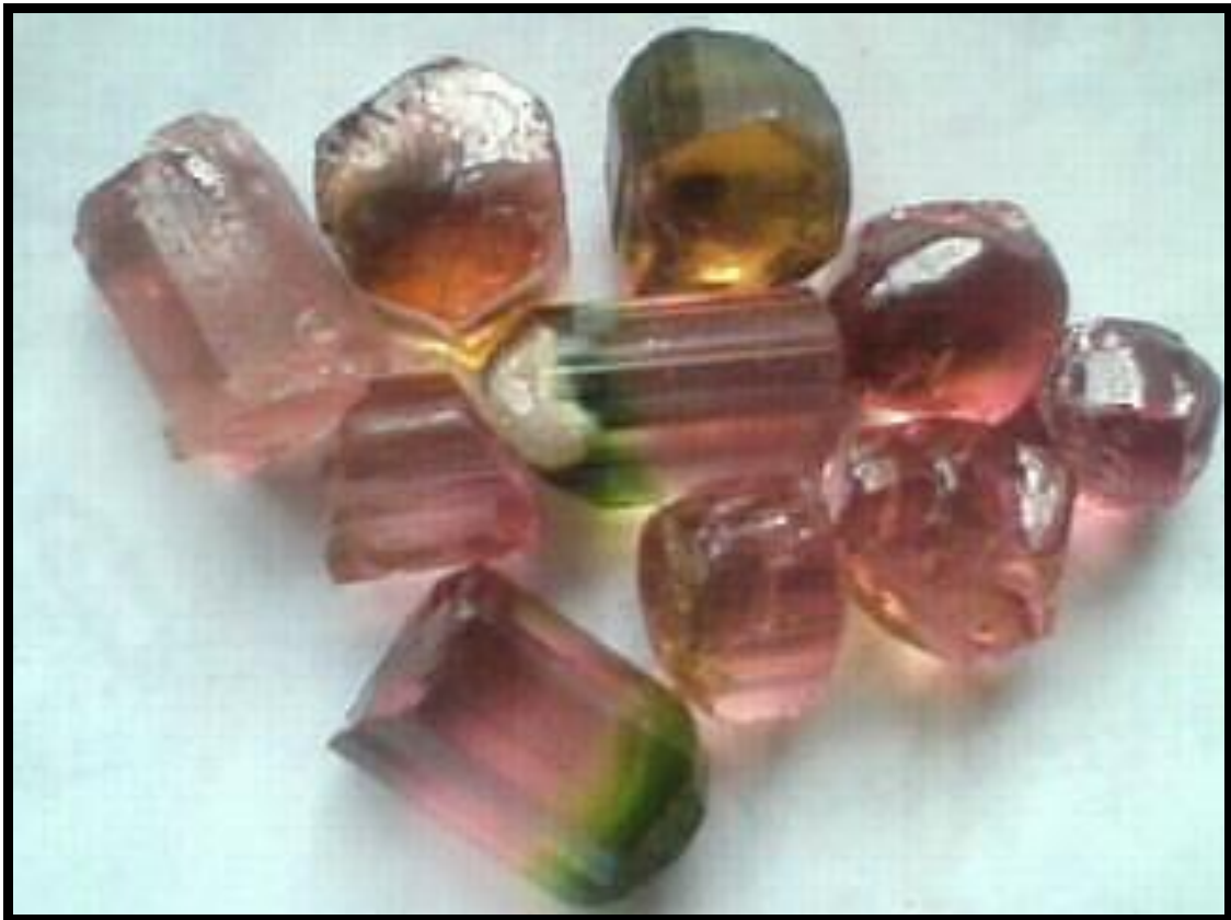
Plate XXIV: Crystals of tourmaline (elbaite) with green cap extracted from cavity in the lepidolite - albite unit, Angwan Doka area.
