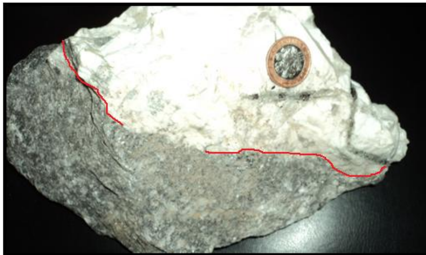
Plate XVI: Hand specimen of border zone of pegmatite composed of albite containing biotite, schorl and Ta oxide minerals abuts the granodiorite, Angwan Doka
