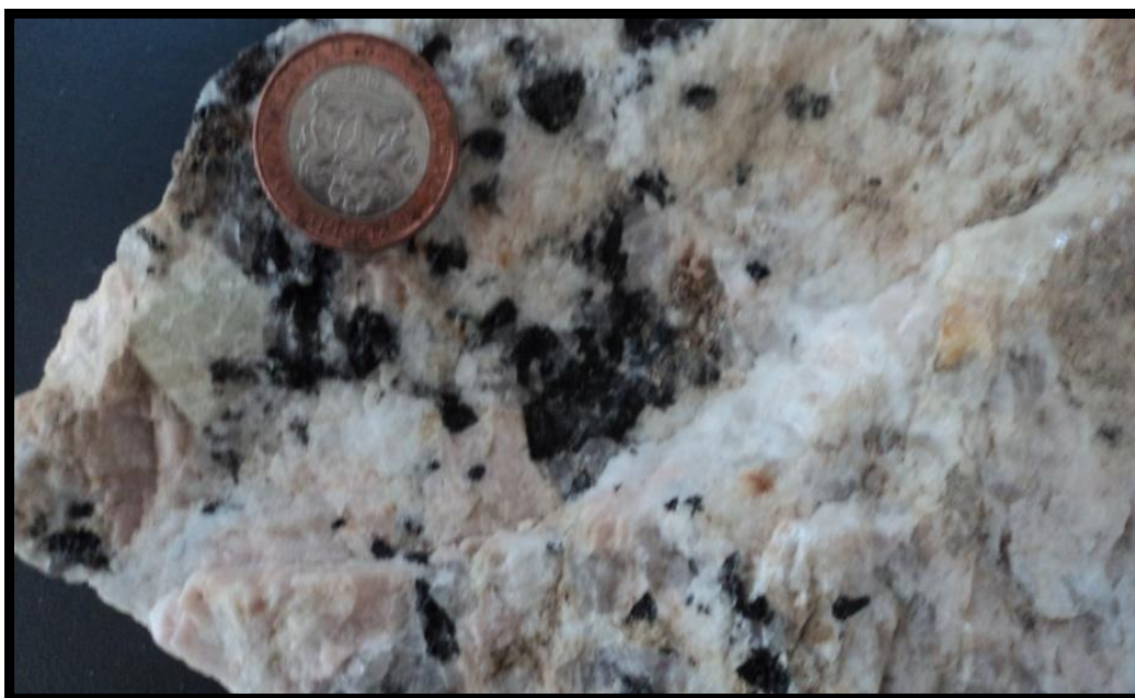
Plate XVII: Photograph of hand specimen from the pegmatite wall zone, Angwan Doka. The rock is composed K-feldspar, albite, graphic intergrowth of quartz and tourmaline with beryl and Ta-oxide mineral.
