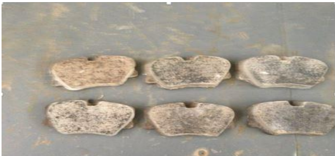
Photograph of the Developed Brake Pad for Mercedes Benz 230E
