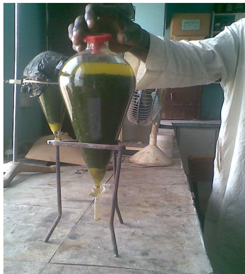
Plate XI: Apparatus for extraction of plant material using the cold maceration method
