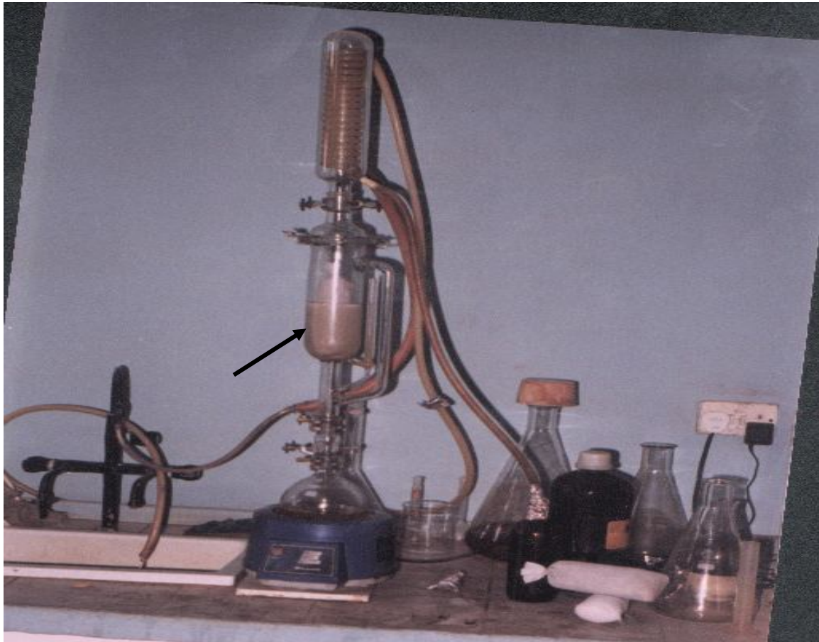
Plate 3.1 Soxhlet apparatus (Quick fit corning Ltd. A division of Stafford England) used for the extraction of plant material
