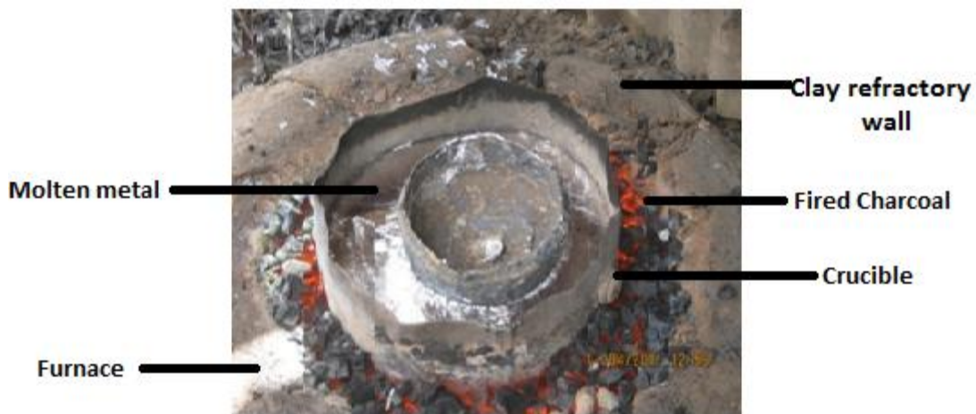
PLATE 1.2 a typical old type crucible furnace used in the foundries. Source: Muchia Market 4/11/2011
