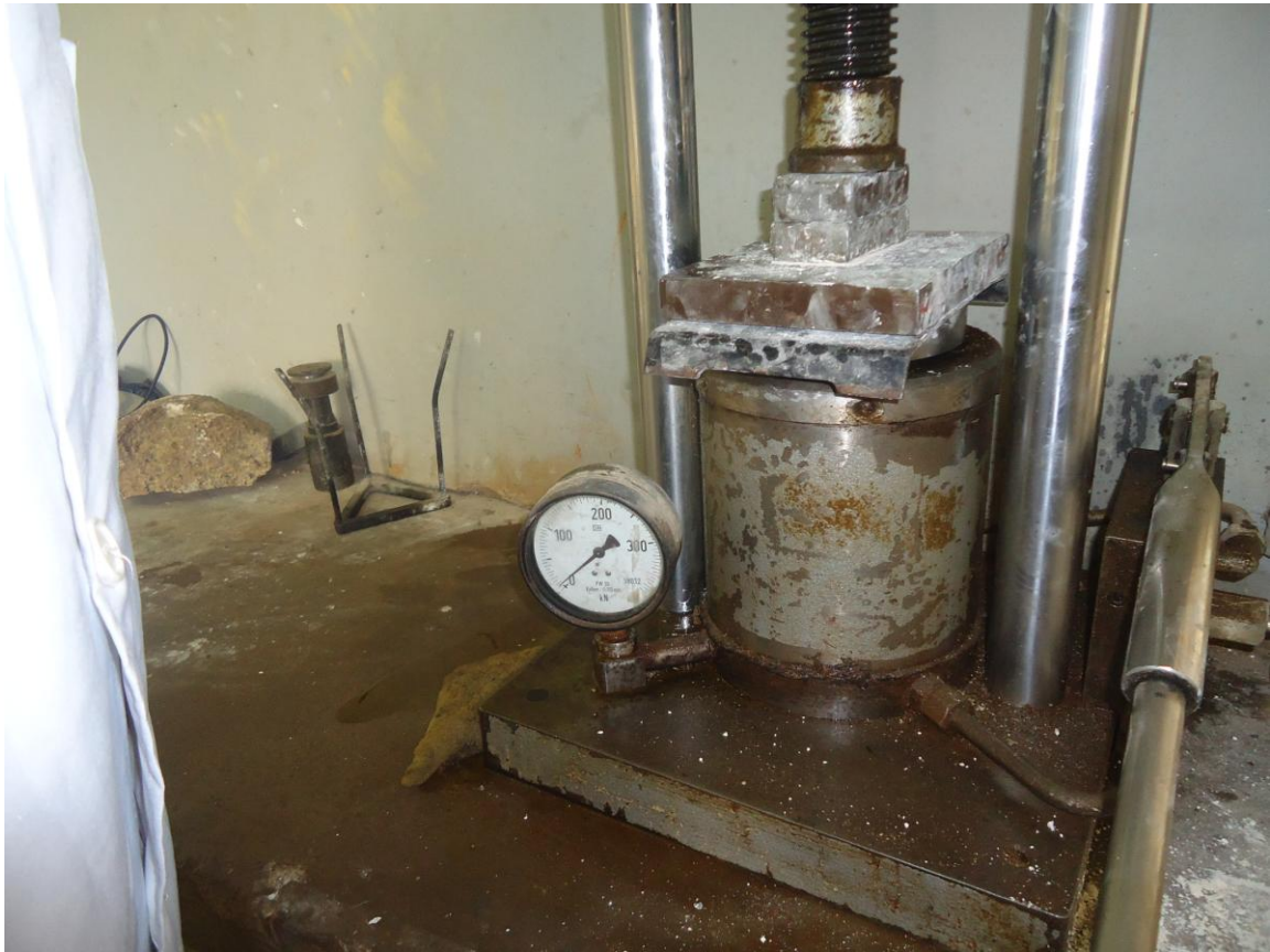
Plate II: Semi-Dry Pressing of the Brick Samples with Hydraulic Pressing Machine
