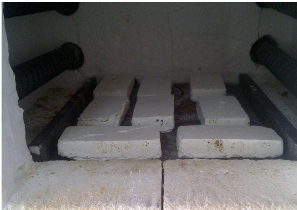
Plate IV: Final Brick Samples in the Furnace
