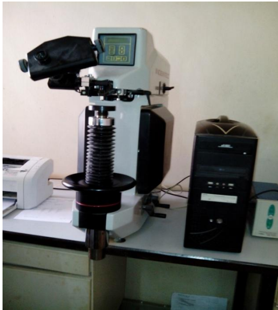
Plate VIII: Indentec Universal Hardness Testing Machine (Metallurgical and Materials Engineering Department, ABU, Zaria).
