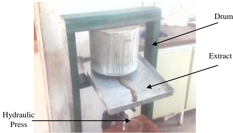
Plate IV: Cold Pressing Set up (National Research Institute for Chemical Technology)
