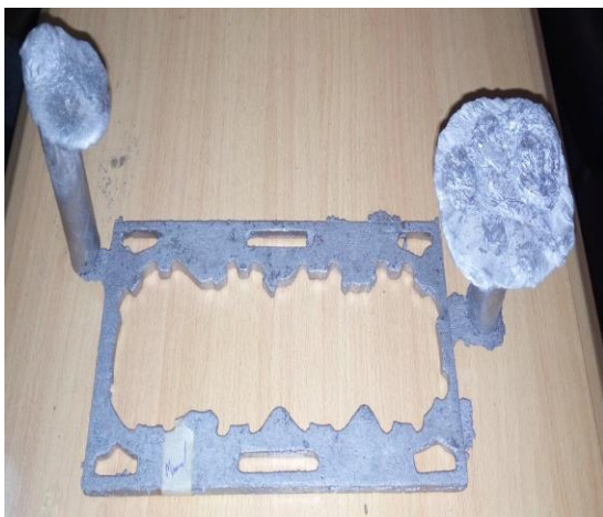
Plate 4.7: Cope side of the water jacket cast using hand-shank ladle pouring
