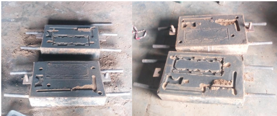
Plate 3.2a: Sand mould for pouring ladle Plate 3.2b: Sand mould for hand-shank ladle
