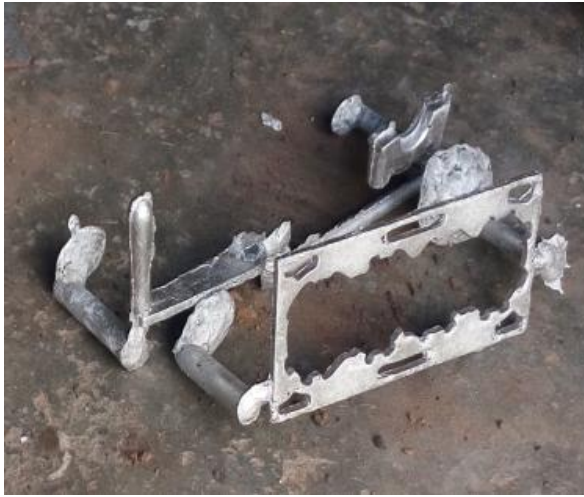
Plate 3.3: Cast sample of improved casting pouring ladle
