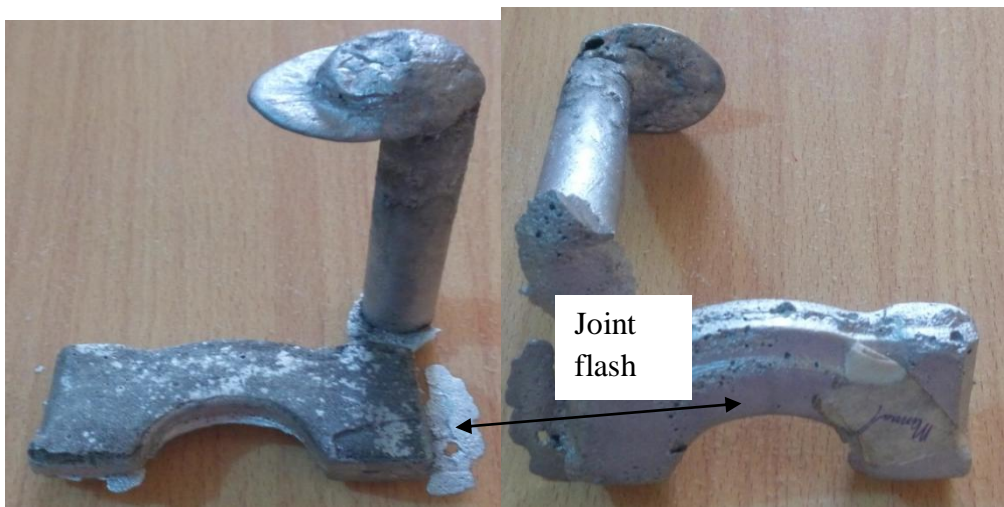
Plate 4.11: Cope side of the bearing cap Plate 4.12: Drag side of the bearing cap cast using hand-shank ladle pouring cast using hand-shank ladle pouring
