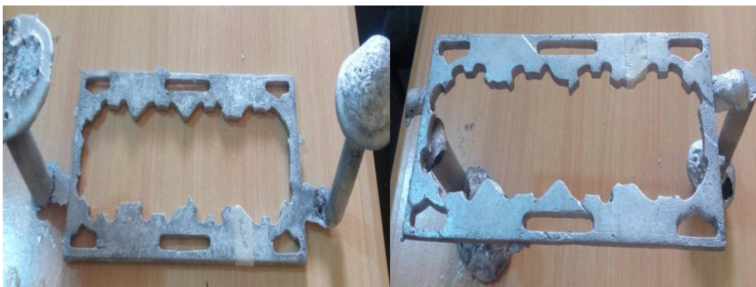
Plate 4.1: Cope side of the water jacket Plate 4.2: Drag side of the water jacket cast using ladle machine pouring cast using ladle machine pouring
