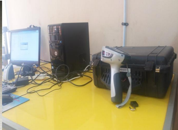
Plate 3.8: Using the XRF machine model XL3t 950 for snap capturing of the sample
