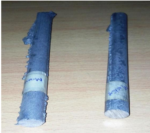
Plate 3.7: Samples for XRF test. XL3t 950 for snap capturing of the sample
