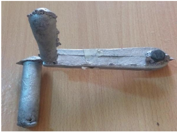
Plate 4.3: Front side of the crank lever cast using ladle machine pouring
