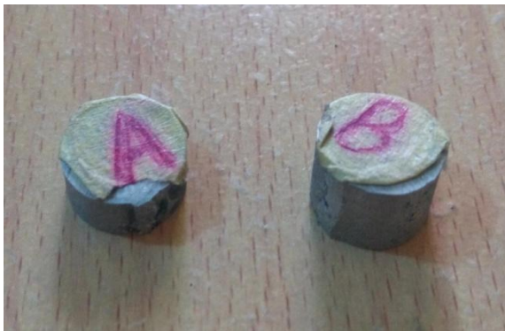
Plate 3.5: Samples for metallography test. Where sample A was from pouring ladle model NJF-1 for snap capturing of the samples and sample B from hand-shank ladle
