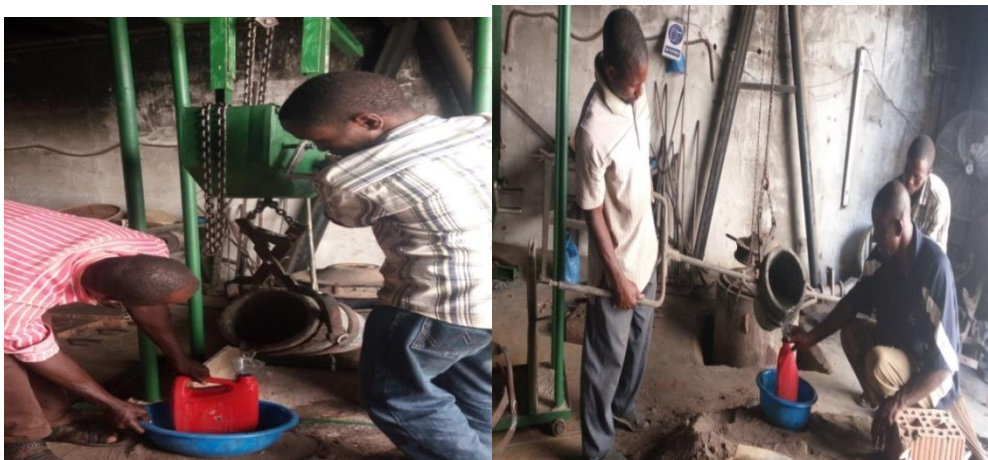
Plate V: Using the pouring ladle for performance evaluation using water
