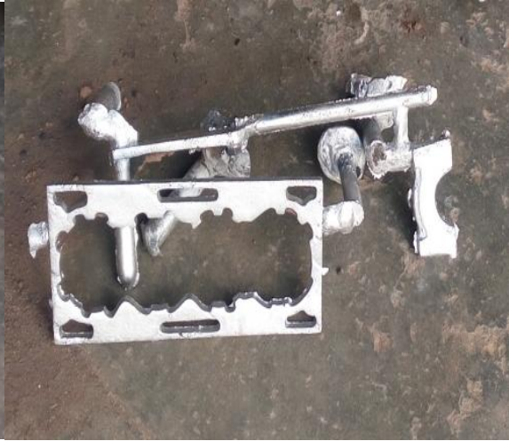
Plate 3.4: Cast sample of hand-shank ladle
