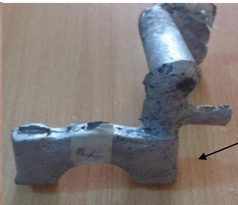
Plate 4.6: Drag side of the bearing cap cast using ladle machine pouring
