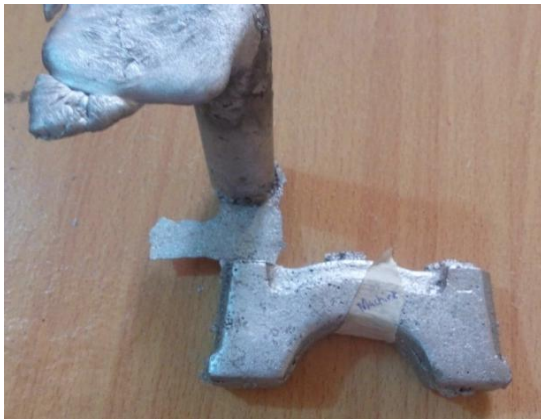
Plate 4.5: Cope side of the bearing cap cast using ladle machine pouring
