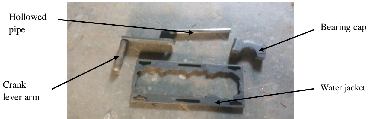
Plate 3.1: Patterns used for the production of mould for the casting
