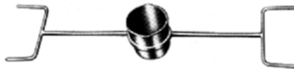
Figure 2.1: Hand-shank casting ladle (Niraj, 2013)
